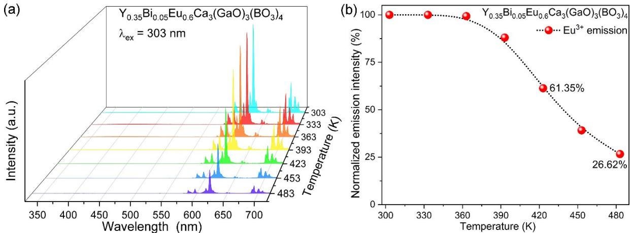
**Fig. S3.** (a) Temperature-dependent PL emission spectra for  $\text{Y}_{0.35}\text{Bi}_{0.05}\text{Eu}_{0.6}\text{Ca}_3(\text{GaO})_3(\text{BO}_3)_4$  under the irradiation of 303 nm and (b) the normalized emission intensity of Eu<sup>3+</sup>.
