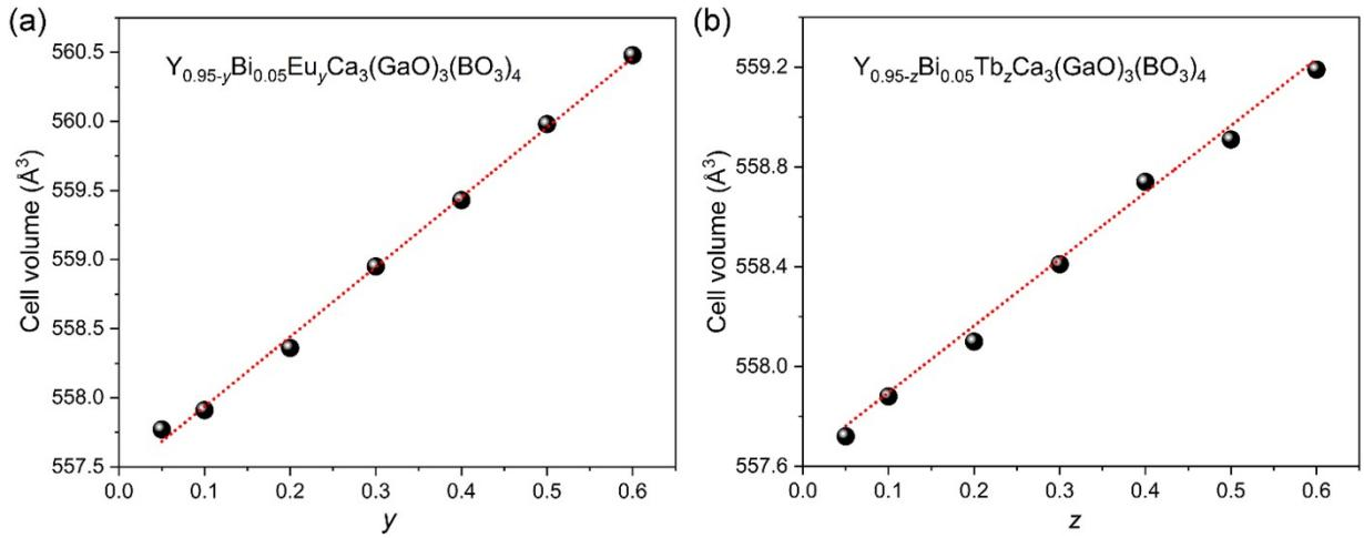
**Fig. S1.** Plot of unit cell volume for (a)  $\text{Y}_{0.95-y}\text{Bi}_{0.05}\text{Eu}_y\text{Ca}_3(\text{GaO})_3(\text{BO}_3)_4$  ( $0.05 \leq y \leq 0.6$ ), (b)  $\text{Y}_{0.95-z}\text{Bi}_{0.05}\text{Tb}_z\text{Ca}_3(\text{GaO})_3(\text{BO}_3)_4$  ( $0.05 \leq z \leq 0.6$ ) obtained from Le Bail fitting.
