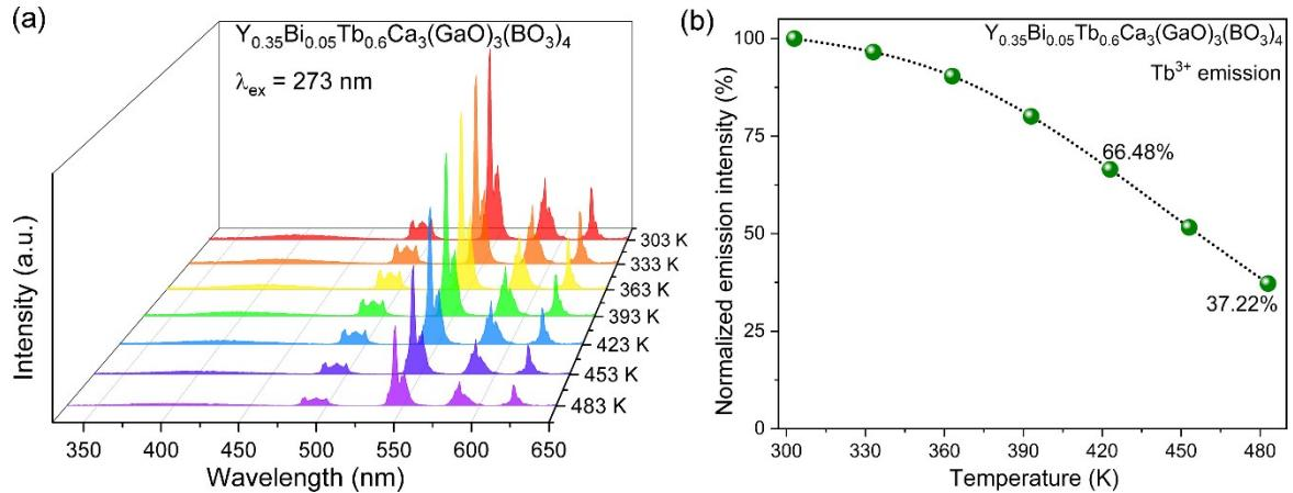
**Fig. S2.** (a) Temperature-dependent PL emission spectra for  $\text{Y}_{0.35}\text{Bi}_{0.05}\text{Tb}_{0.6}\text{Ca}_3(\text{GaO})_3(\text{BO}_3)_4$  under the irradiation of 273 nm and (b) the normalized emission intensity of Tb<sup>3+</sup>.
