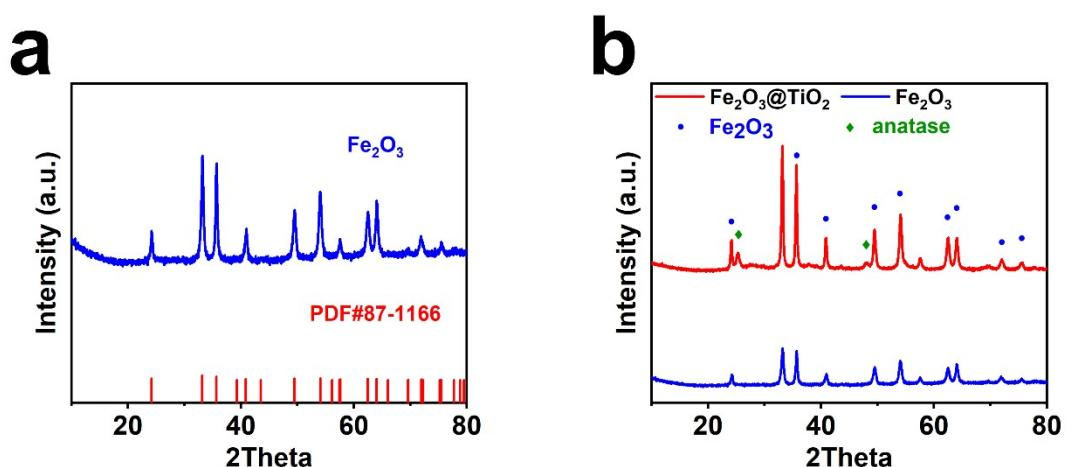
Fig. S2. XRD patterns of (a)  $\text{Fe}_2\text{O}_3$  nanocube, (c-d)  $\text{Fe}_2\text{O}_3@\text{TiO}_2$  nanocube.
