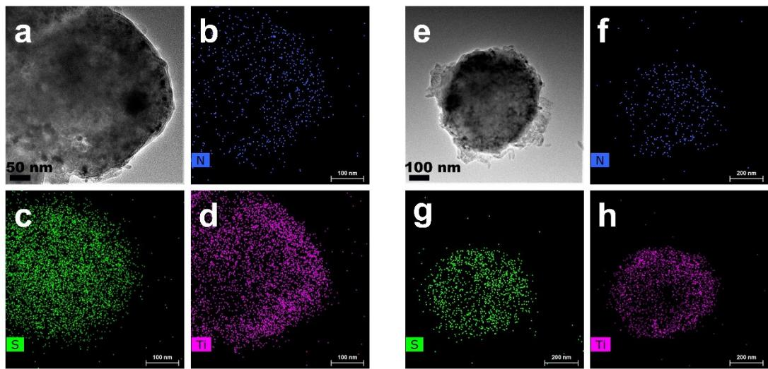
Fig. S7. (a-d) The existence of the polysulfides in the electrodes in the middle of charge, (e-h) The existence of the polysulfides in the electrodes in the middle of discharge.
