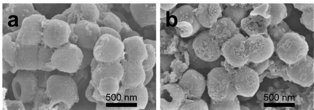
Fig. S8. (a-b) SEM image of S/TiN@C NCs after 200 cycles at 0.5 C.
