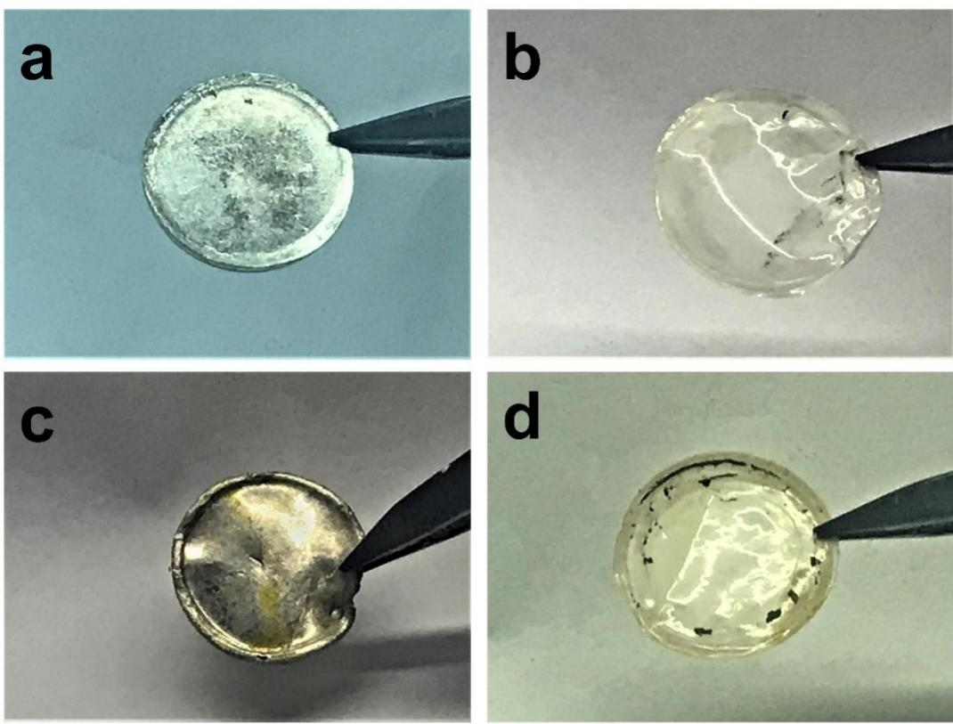
Fig. S9. (a-b) The optical photos of lithium plate and separator in the battery based on S/TiN@C electrode after 200 cycles at 0.5 C, (c-d) The optical photos of lithium plate and separator in the battery based on S/C electrode after 200 cycles at 0.5 C.
