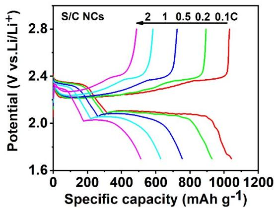
Fig. S6. Charge–discharge curves of S/C NCs cathode at different rates.
