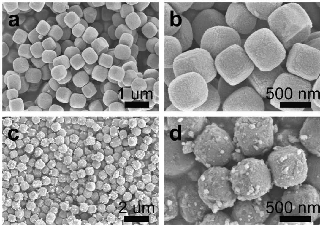
Fig. S1. SEM images of (a-b)  $\text{Fe}_2\text{O}_3$  nanocube, (c-d)  $\text{Fe}_2\text{O}_3@\text{TiO}_2$  nanocube.
