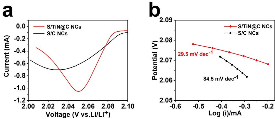
Fig. S5. (a) Details obtained from CV curves, (b) Tafel plots calculated from the CV reduction peak at 2.05 V.
