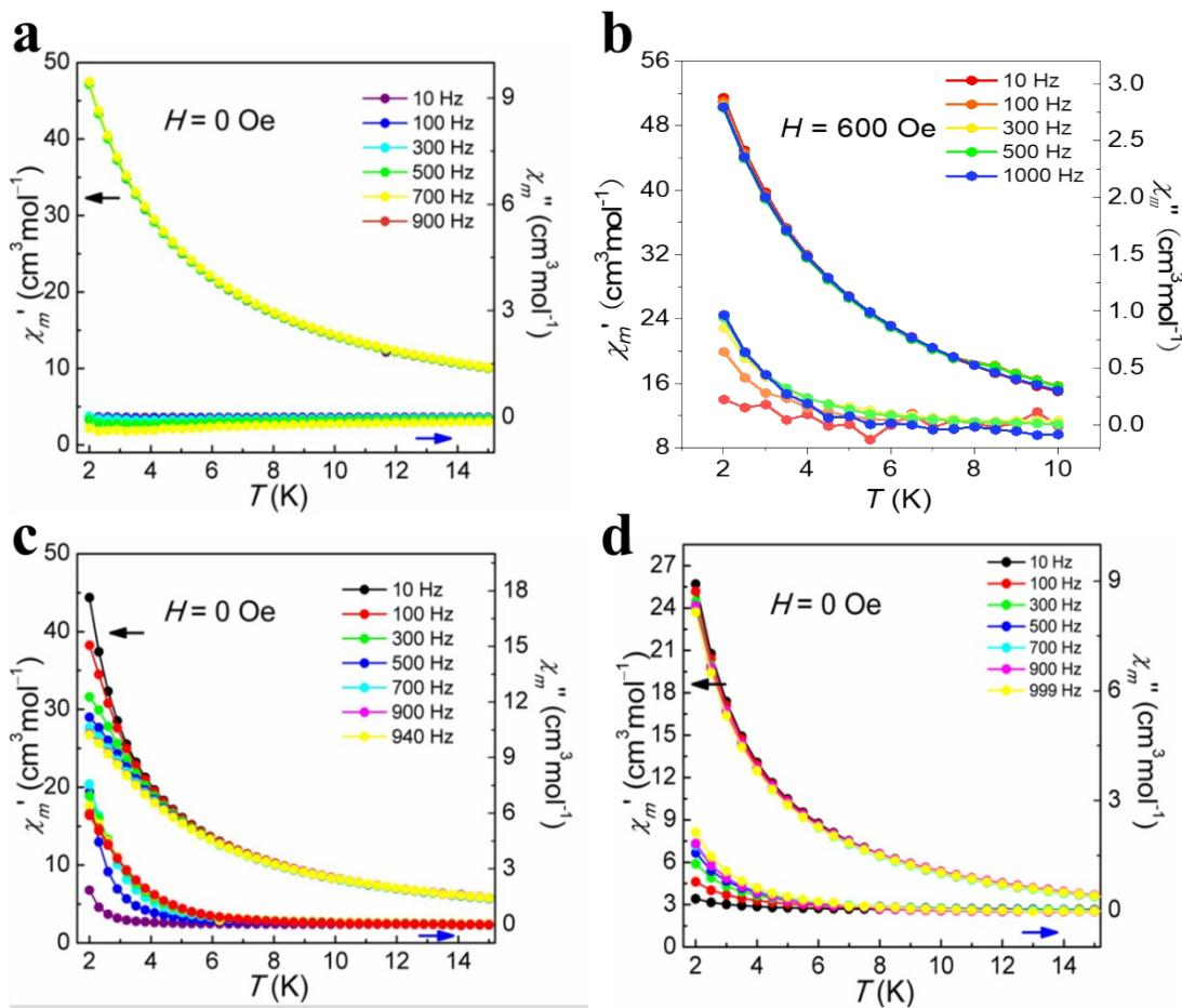
**Figure S9.** Temperature-dependent  $\chi'$  and  $\chi''$  AC susceptibilities under 0 and 600 Oe DC fields for cluster **1** (a and b); temperature-dependent  $\chi'$  and  $\chi''$  AC susceptibilities under 0 Oe DC fields for clusters **2-3** (c and d).
