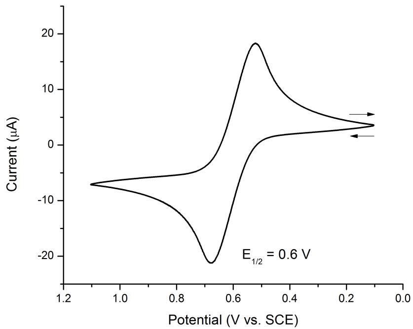
**Figure S9.** Cyclic Voltammogram of **2** with 0.1M  $[\text{N}(n\text{Bu})_4]\text{PF}_6$  in DCM (1mM) as referenced to decamethylferrocene (internal standard, adjusted to SCE).
