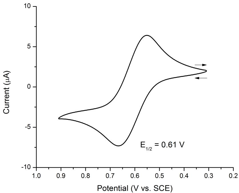
**Figure S10.** Cyclic Voltammogram of **5** with 0.1M  $[\text{N}(n\text{Bu})_4]\text{PF}_6$  in DCM (1mM) as referenced to decamethylferrocene (internal standard, adjusted to SCE).
