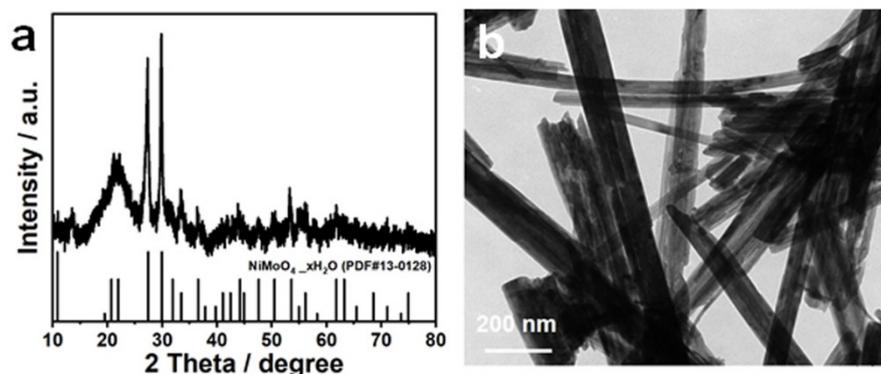
**Fig. S1** (a) XRD pattern and (b) TEM image of the as-synthesized NiMoO<sub>4</sub> precursor by the hydrothermal reaction between Ni(NO<sub>3</sub>)<sub>2</sub> and Na<sub>2</sub>MoO<sub>4</sub>.
