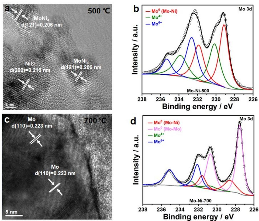
**Fig. S3** HRTEM images and Mo 3d XPS spectra of the products of NiMoO<sub>4</sub> reduction transformation at 500 °C (a, b) and 700 °C (c, d).
