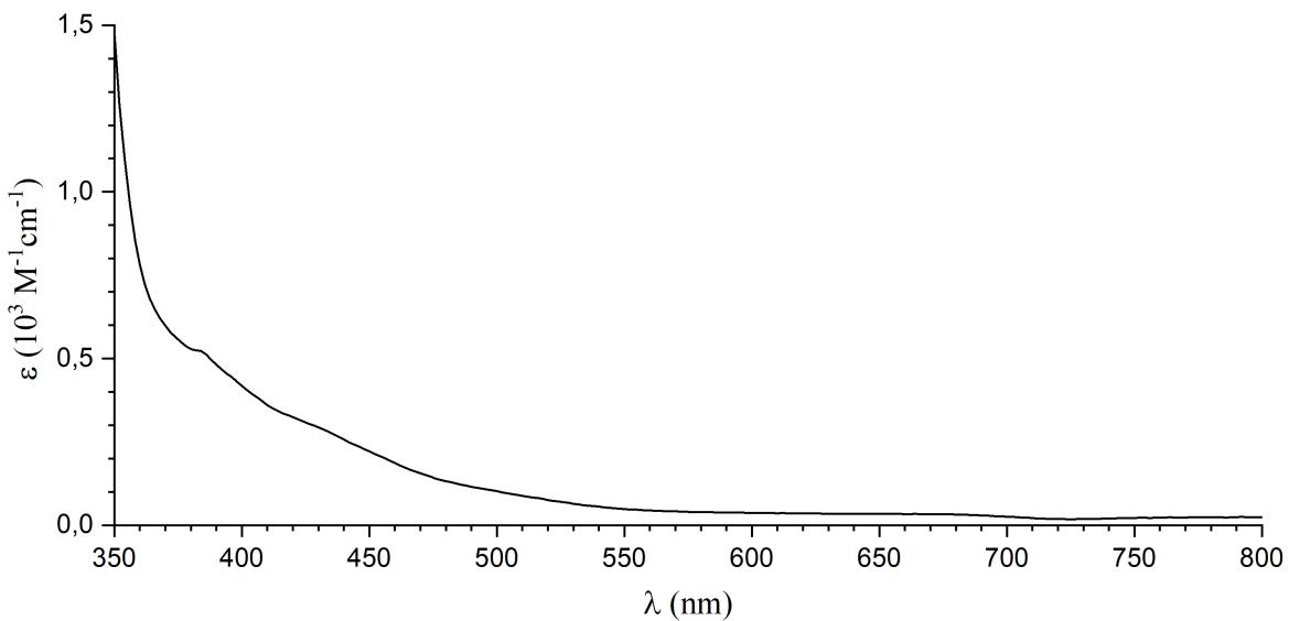
**Figure S7.** Experimental UV-visible spectrum of a mixture of  $\text{Cp}^*_2\text{Sm(THF)}_2$  (2 eq) and  $\text{Me}_2\text{DBA}$  (1 eq) in toluene after exposure to  $\text{N}_2$  overnight.
