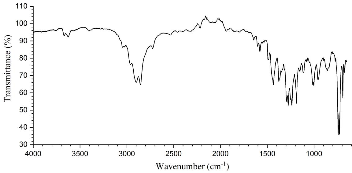
**Figure S5.** IR spectrum of the reaction mixture between  $[(\text{C}_5\text{Me}_5)_2\text{Sm}(\text{THF})_2][(\text{C}_5\text{Me}_5)_2\text{Sm}(\eta_2\text{-N}_2\text{B}_2\text{C}_{14}\text{H}_{14})]$  and  $\text{MeI}$ .
