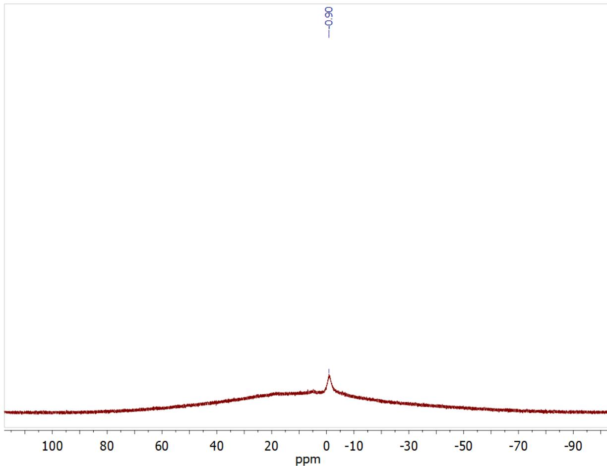
**Figure S2.**  $^{11}B$  NMR spectrum taken in  $C_6D_6$  after  $(C_5Me_5)_2Sm(THF)_2$  (2 eq) was reacted with 9,10-Me<sub>2</sub>-9,10-diboraanthracene ( $B_2Me_2$ , 1 eq) in toluene at  $-78\text{ }^\circ C$  under  $N_2$  overnight.
