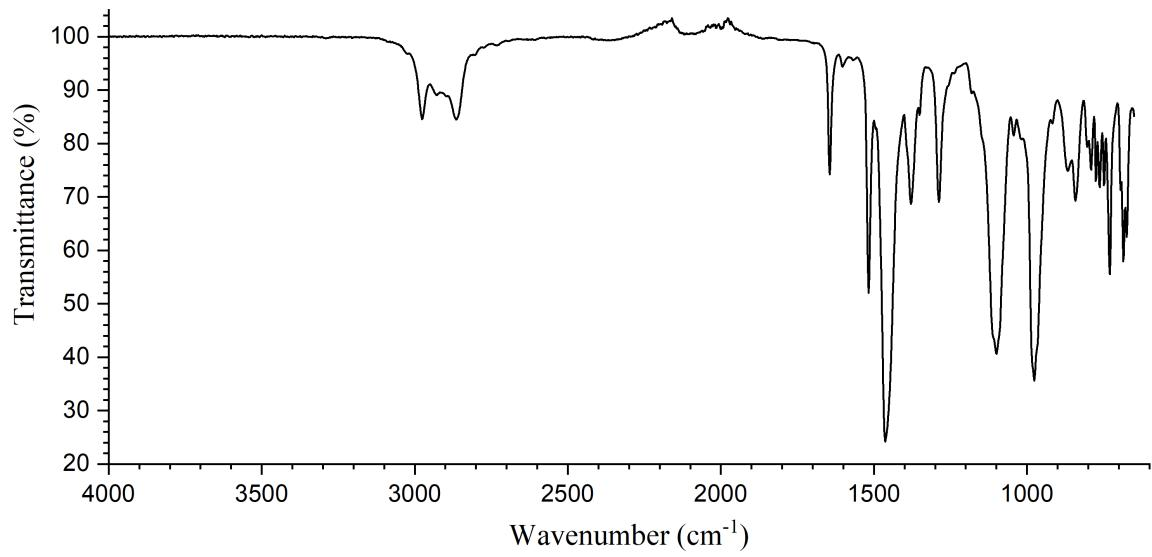
**Figure S4.** IR spectrum of the reaction mixture between  $(\text{C}_5\text{Me}_5)_2\text{Sm}(\text{THF})_2$  and  $\text{B}(\text{C}_6\text{F}_5)_3$ .
