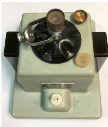
Fig. S57. Narva DDR GM 9458 vibration ball mill with a custom-built agate insert
