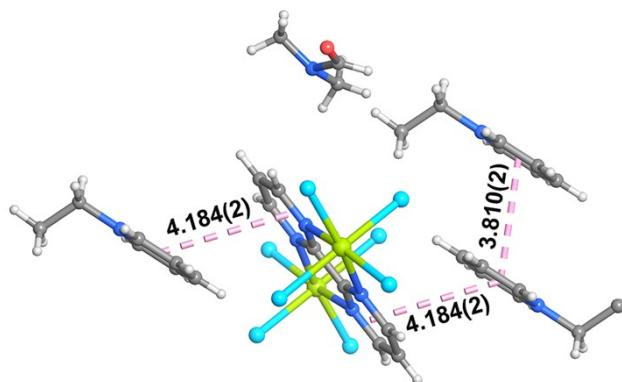
**Figure S4**  $\pi-\pi$  interactions shown in rose dotted lines for **1**. The ring-to-ring distances are 3.810(2) and 4.184(2) Å.
