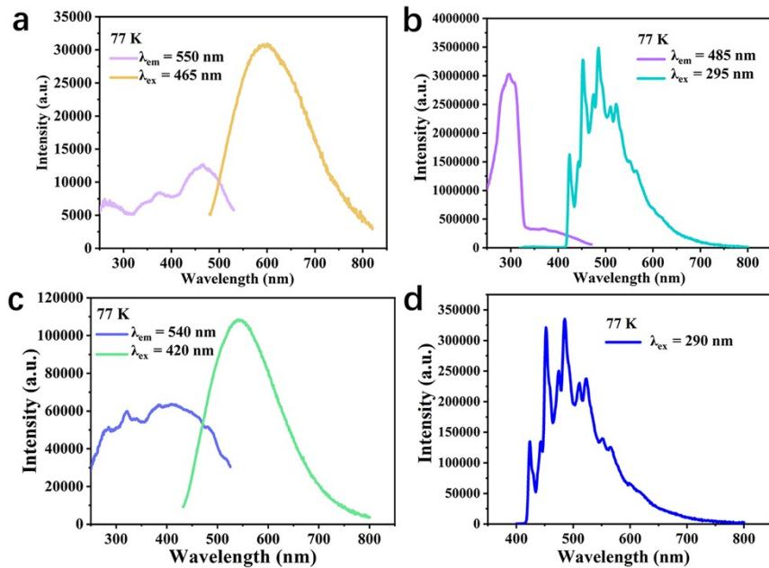
**Figure S15** The PLE and PL spectra at 77 K for **1** (a), **2** (b) and **3** (c). The PL spectrum of **1-h** at 77 K. Note that the PL spectra for **2** and **1-h** at 77 K are comparable except the difference in PL intensity.
