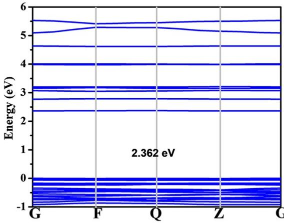
**Figure S11** The electronic band structure of **3**. The calculated bandgap of **3** is 2.362 eV.
