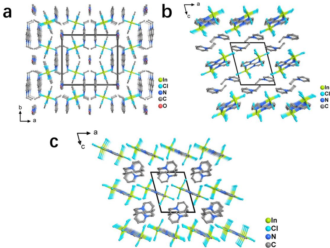
**Figure S3** View of structural packing modes for **1** (a) along the  $c$  axis, **2** (b) along the  $b$  axis and **3** (c) along the  $b$  axis. H atoms are omitted for clarity.
