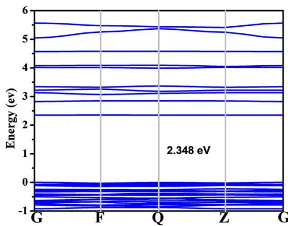
**Figure S10** The electronic band structure of **2**. The calculated bandgap of **2** is 2.348 eV.
