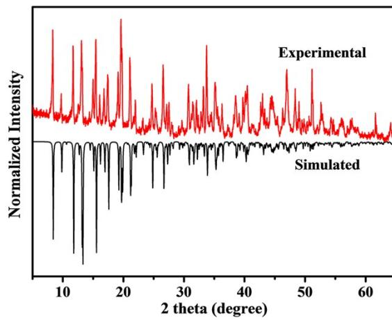
**Figure S6** Experimental and simulated PXRD patterns of **2**.
