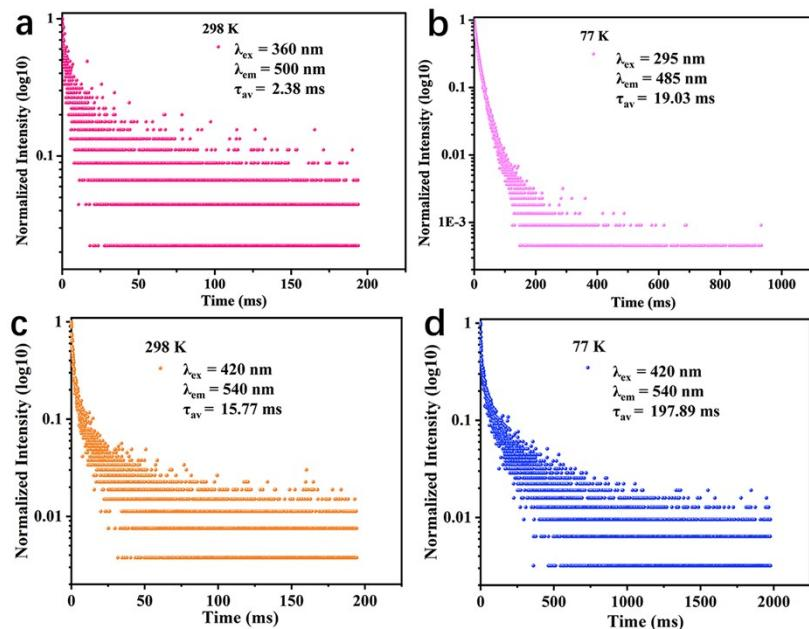
**Figure S16** The PL decay spectra of **2** at 298 K (a) and at 77 K (b) and of **3** at 298 K(c) and at 77 K (d).
