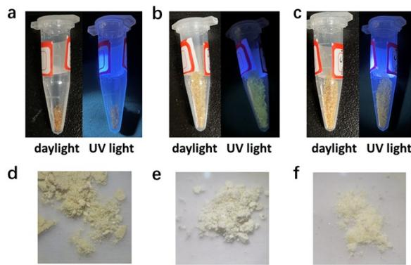
**Figure S9** Photographs of crystals under daylight (left) and UV irradiation (right) for **1** (a), **2** (b) and **3** (c). Photographs of powdered samples obtained by grinding crystals **1** (d), **2** (e) and **3** (f).
