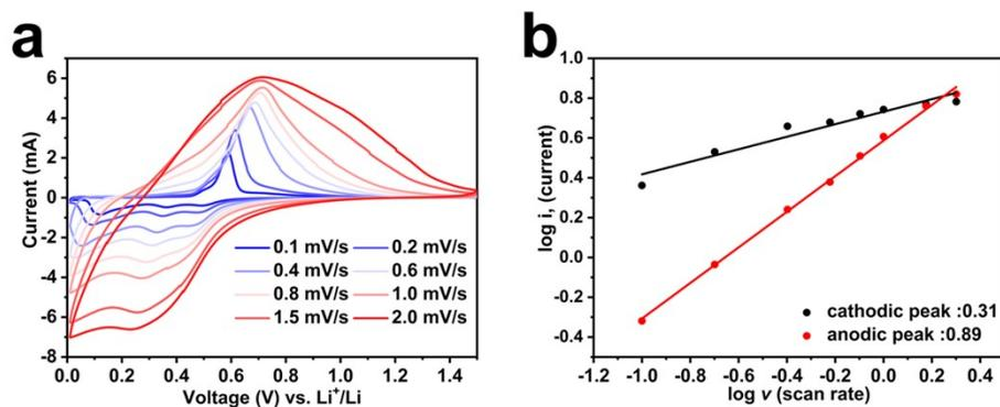
**Figure S6.** (a) Curves at various scan rates from 0.1 to 2 mV s<sup>-1</sup>. (b) log (i) versus log (v) plots and b value for the slope.
