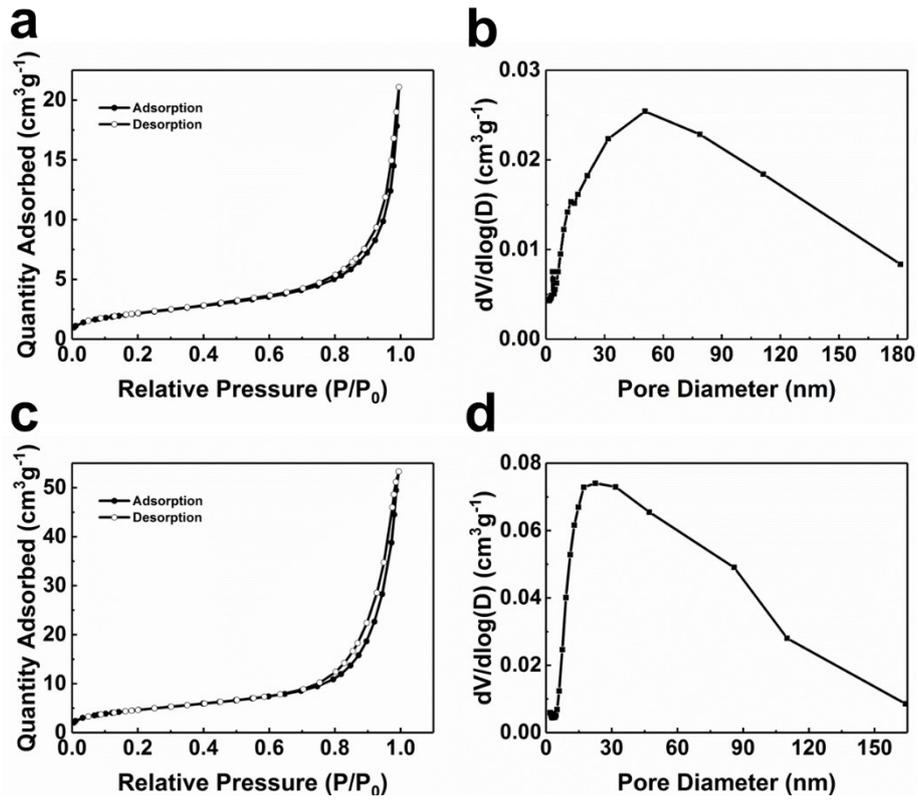
**Figure S10.** (a)  $\text{N}_2$  adsorption-desorption isotherms and (b) the pore-size distribution calculated from the desorption branch of the nanoporous Z-Si materials. (c)  $\text{N}_2$  adsorption-desorption isotherms and (d) the pore-size distribution calculated from the desorption branch of the nanoporous A-Si materials.
