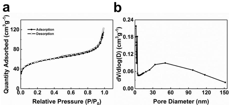
**Figure S4.** (a) N<sub>2</sub> adsorption-desorption isotherms and (b) the pore-size distribution calculated from the desorption branch of the nanoporous A-Ge materials.
