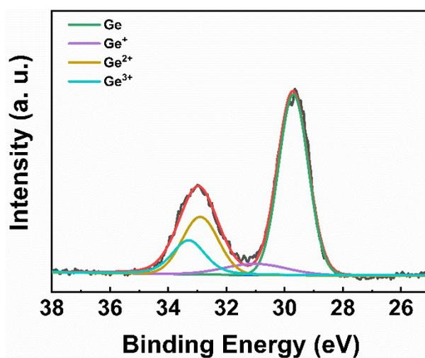
**Figure S3.** XPS spectra of Ge 3d of nanoporous A-Ge materials.
