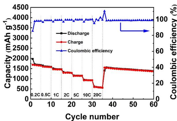
**Figure S11.** The rate capability of nanoporous Z-Si materials.
