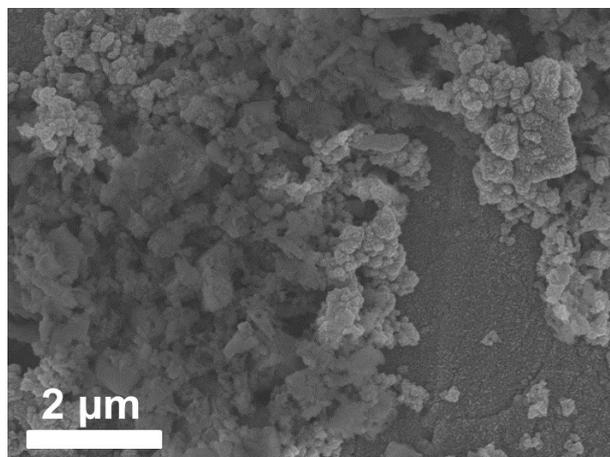
**Figure S9.** SEM image of the nanoporous A-Si materials.
