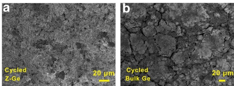
**Figure S7.** FESEM images of (a) Z-Ge and (b) bulk Ge electrodes after 100 cycles.
