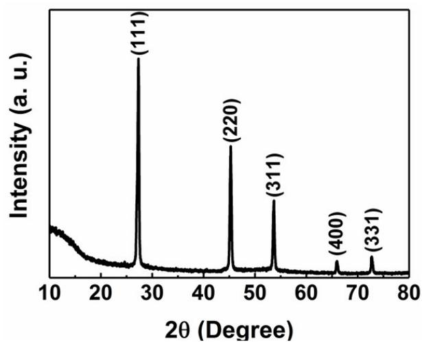
**Figure S1.** XRD patterns of the nanoporous A-Ge materials.
