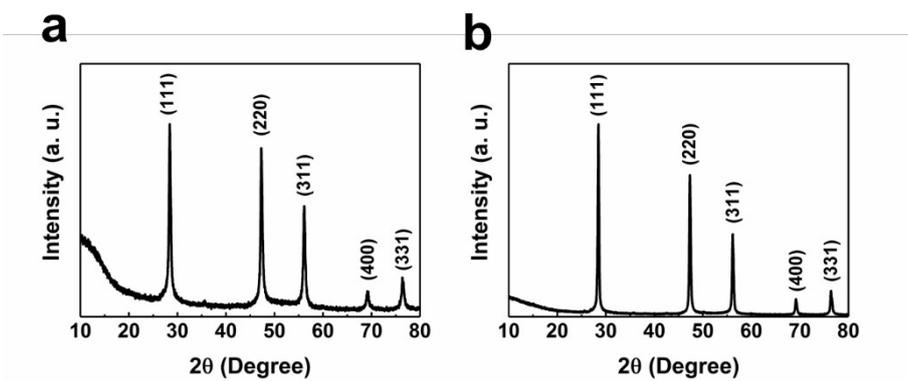
**Figure S8.** XRD patterns of the nanoporous Z-Si (a) and A-Si (b) materials.
