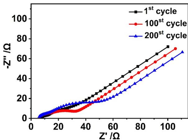
**Figure S5.** Electrochemical impedance spectra (EIS) of Z-Ge materials.
