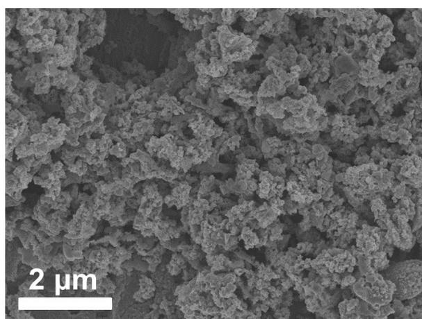
**Figure S2.** SEM image of the nanoporous A-Ge materials.
