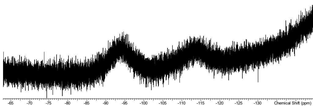
Figure S11.2.2  $^{19}\text{F}\{^1\text{H}\}$  NMR spectrum  $\text{CD}_2\text{Cl}_2$ , 213 K; \* =  $[\text{GeF}_4\{\kappa^1\text{-P}(\text{CH}_2\text{CH}_2\text{PPh}_2)_3\}_2]$ , ^ = unidentified impurity
