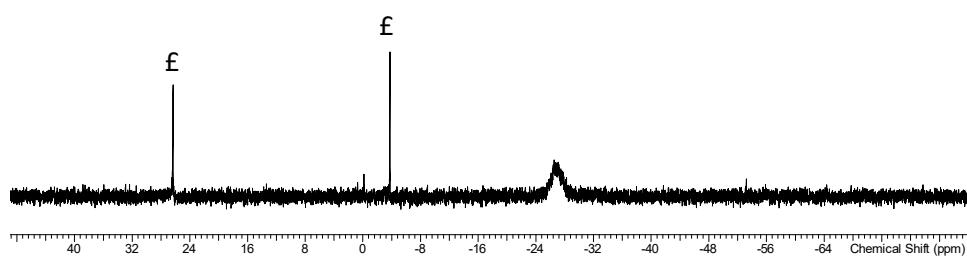
Figure S7.3.2  $^{31}\text{P}\{\text{H}\}$  NMR spectrum  $\text{CD}_2\text{Cl}_2$ , 183 K; \*=  $[\text{GeF}_4\{o\text{-C}_6\text{H}_4(\text{PMe}_2)_2\}]$
