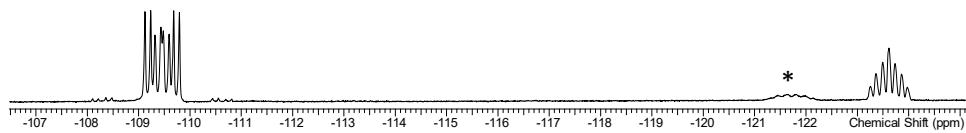
Figure S7.3.1  $^{31}\text{P}\{\text{H}\}$  NMR spectrum  $\text{CD}_2\text{Cl}_2$ , 298 K;  $\ddagger$ = unidentified impurities
