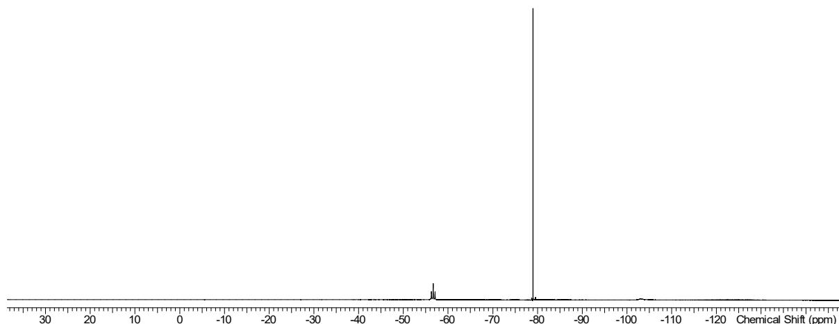
Figure S6.3  $^{31}\text{P}\{^1\text{H}\}$  NMR spectrum  $\text{CD}_2\text{Cl}_2$ , 298 K; \* =  $[\text{HP}^{\text{i}}\text{Pr}_3]^+$
