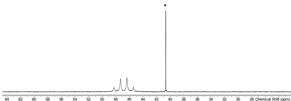
Figure S6.3.2  $^{31}\text{P}\{^1\text{H}\}$  spectrum  $\text{CD}_2\text{Cl}_2$ , 183 K; \* =  $[\text{HP}^{\text{i}}\text{Pr}_3]^+$
