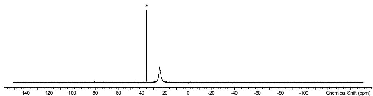
Figure S2.5  $^{31}\text{P}\{\text{H}\}$  NMR spectrum in  $\text{CD}_2\text{Cl}_2$ , 183 K.
