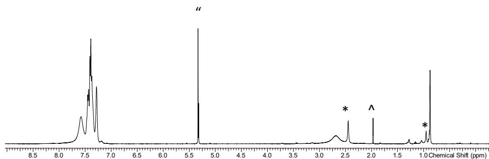
Figure S10.1.2 <sup>1</sup>H NMR spectrum CD<sub>2</sub>Cl<sub>2</sub> 183 K.
