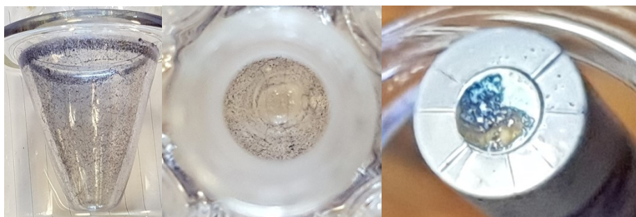
Fig. S28 (Above) CV of Species 1 in dry dichloromethane with 0.1 M TBAPF 6 and 0.3 mM Ferrocene. (Below) Images of the deposit in the electrochemical cell and on the surface of the working electrode
