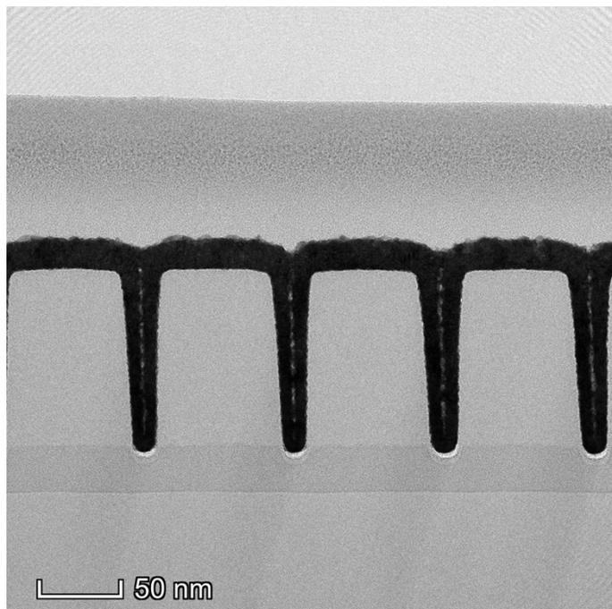
**Figure S16.** TEM images of Re thin film grown on *in-situ* TiN coated structures annealed under H<sub>2</sub> atmosphere (12 Torr, 400 °C, 1 h) followed by heating to 600 °C (Ar, 10 min)
