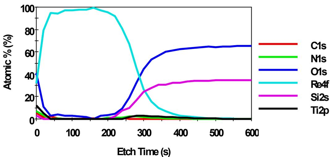
**Figure S15.** XPS spectra of a Re thin film annealed under NH<sub>3</sub> atmosphere (11 Torr, 400 °C, 1 h) followed by heating to 600 °C (Ar, 10 min). The film was about 20 nm thick prior to annealing and was grown at 340 °C.
