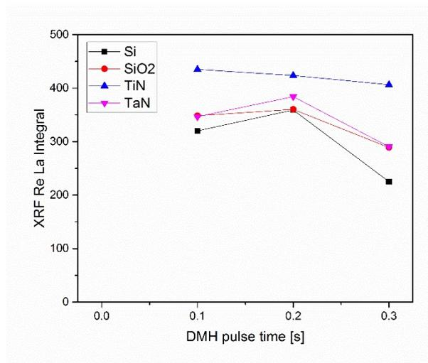
**Figure S5.** XRF counts with respect to the  $\text{Me}_2\text{NNH}_2$  pulse time for films grown at  $340\text{ }^\circ\text{C}$  with 500 cycles.
