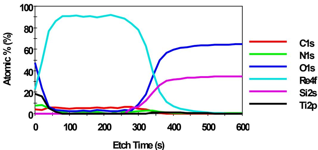
**Figure S14.** XPS spectra of a Re thin film annealed under H<sub>2</sub> atmosphere (12 Torr, 400 °C, 1 h) followed by heating to 600 °C (Ar, 10 min). The film was about 20 nm thick prior to annealing and was grown at 340 °C.
