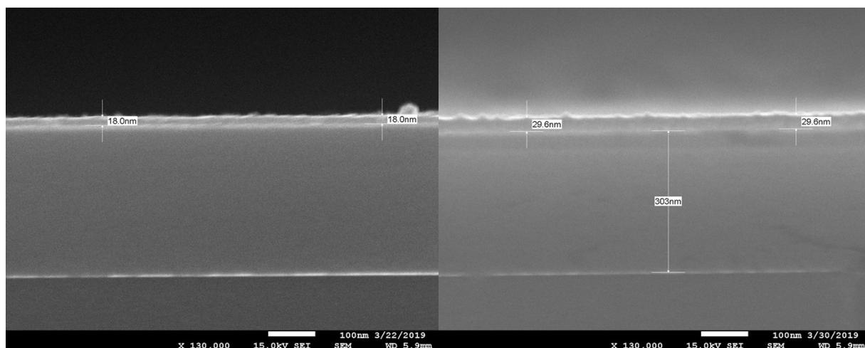
**Figure S8.** SEM cross-sections of Re films grown at 325 °C (left) and 340 °C (right) for 500 cycles.
