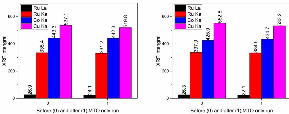
**Figure S2.** XRF counts of the metal substrates before and after MTO only deposition at 340 °C for 500 (left) and 1000 (right) cycles.
