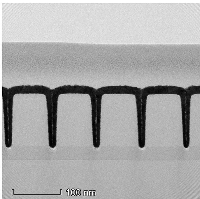
**Figure S17.** TEM images of Re thin film grown on *in-situ* TiN coated structures annealed under NH<sub>3</sub> atmosphere (11 Torr, 400 °C, 1 h) followed by heating to 600 °C (Ar, 10 min)
