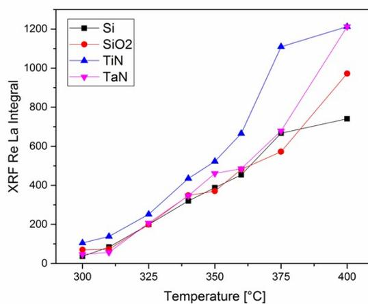
**Figure S6.** XRF counts with respect to the deposition temperature for films grown with 500 cycles.
