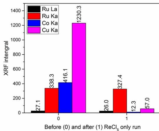
**Figure S3.** XRF counts of the metal substrates before and after ReCl<sub>5</sub> only deposition at 400 °C for 500 cycles.
