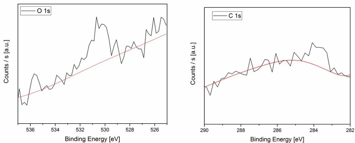
**Figure S12.** High resolution O 1s (left) and C 1s (right) XPS spectra of 70 nm thick Re films grown at 340 °C on Si with native oxide substrate.
