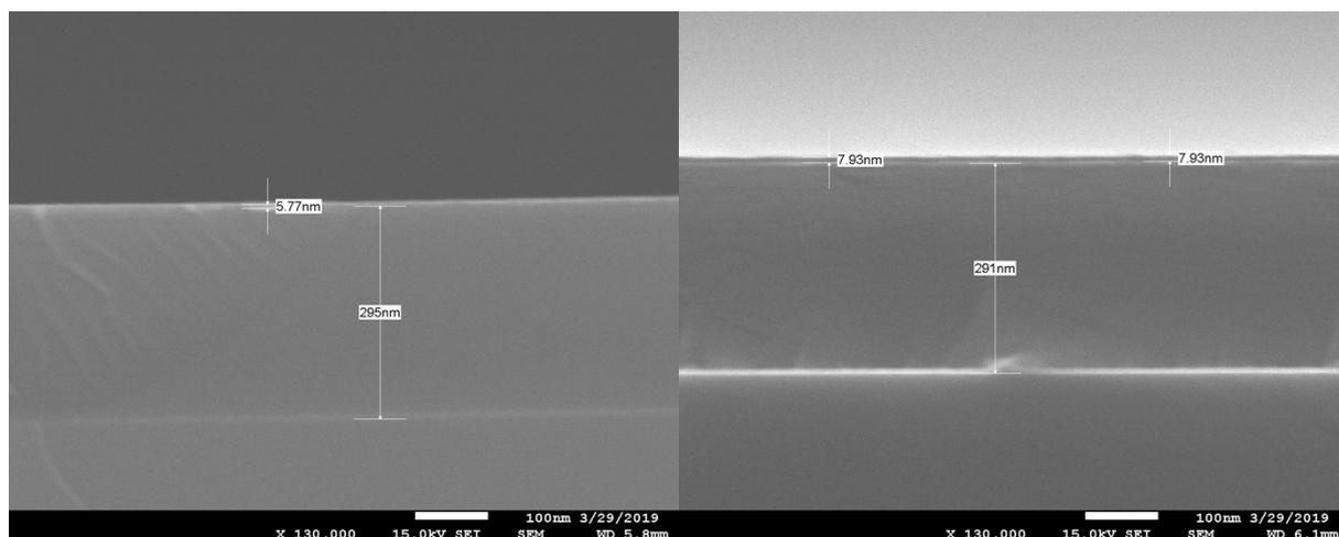
**Figure S7.** SEM cross-sections of Re films grown at 300 °C (left) and 310 °C (right) for 500 cycles.
