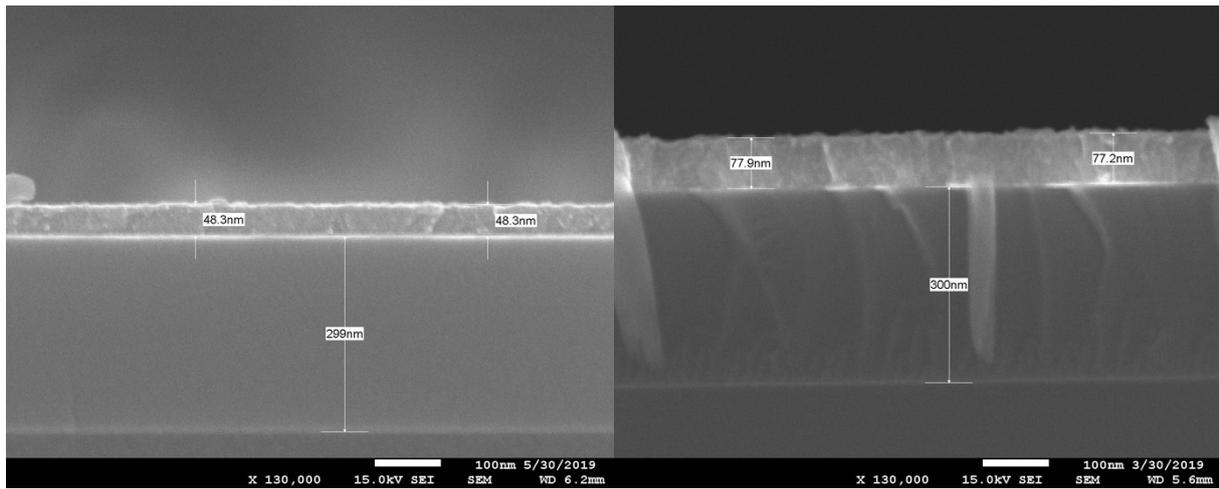
**Figure S10.** SEM cross-sections of Re films grown at 375 °C (left) and 400 °C (right) for 500 cycles.
