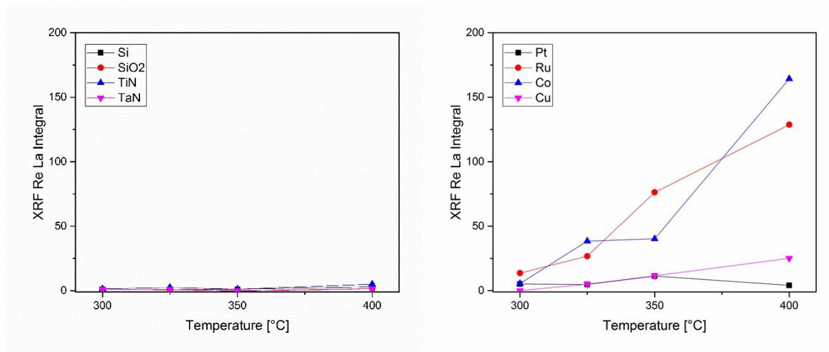
**Figure S1.** MTO self-decomposition behavior with respect to the deposition temperature on insulating (left) and metallic (right) substrate surfaces as evaluated by XRF
