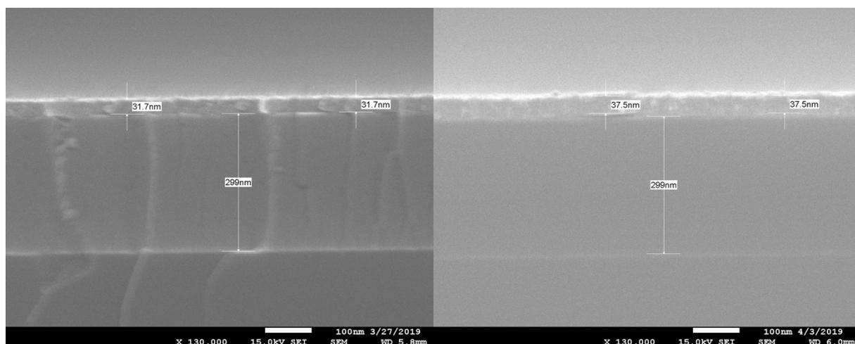
**Figure S9.** SEM cross-sections of Re films grown at 350 °C (left) and 360 °C (right) for 500 cycles.
