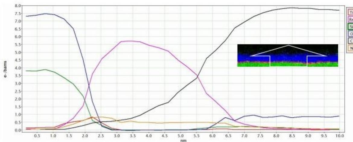
**Figure S13.** EELS spectra of a 3.7 nm Re film grown on 1 nm thick *in situ* TiN layer at 340 °C on SiO<sub>2</sub>.
