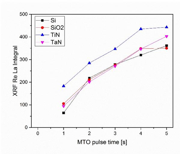
**Figure S4.** XRF counts with respect to the MTO pulse time for films grown at 340 °C with 500 cycles.
