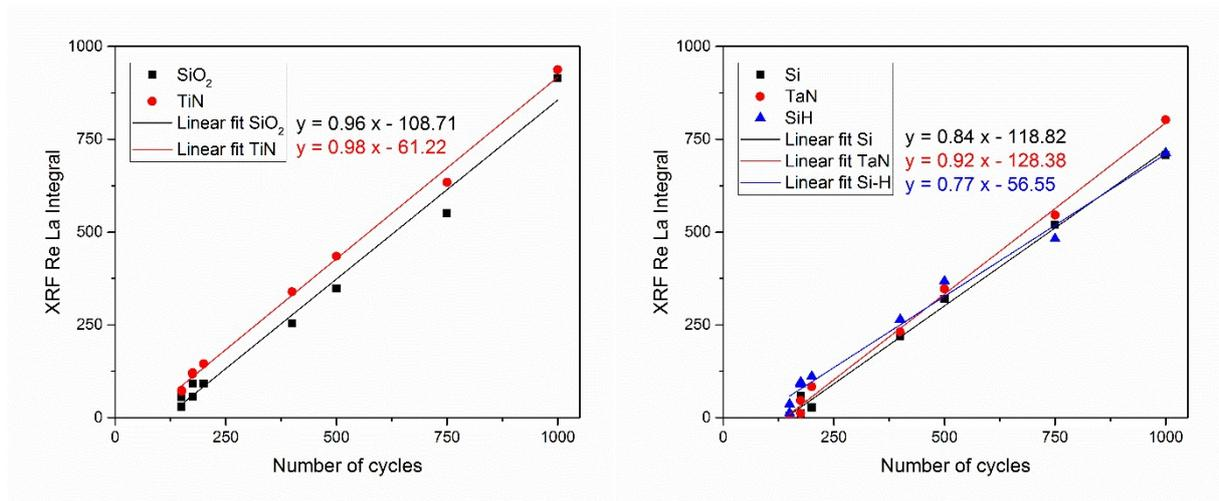
**Figure S11.** XRF counts versus number of cycles for Re films grown at 340 °C on various substrates.
