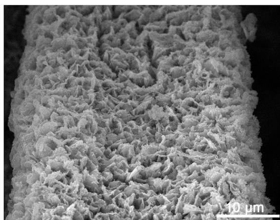
**Fig. S22** SEM image of the CoP-CNT/Ni<sub>2</sub>P/NF catalyst after long-time electrolysis toward OER in 1.0 M KOH.
