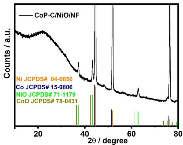
**Fig. S8** The spectrum to contrast the XRD pattern of CoP-C/NiO/NF and the standard card of metallic Co/Ni and CoO/NiO.
