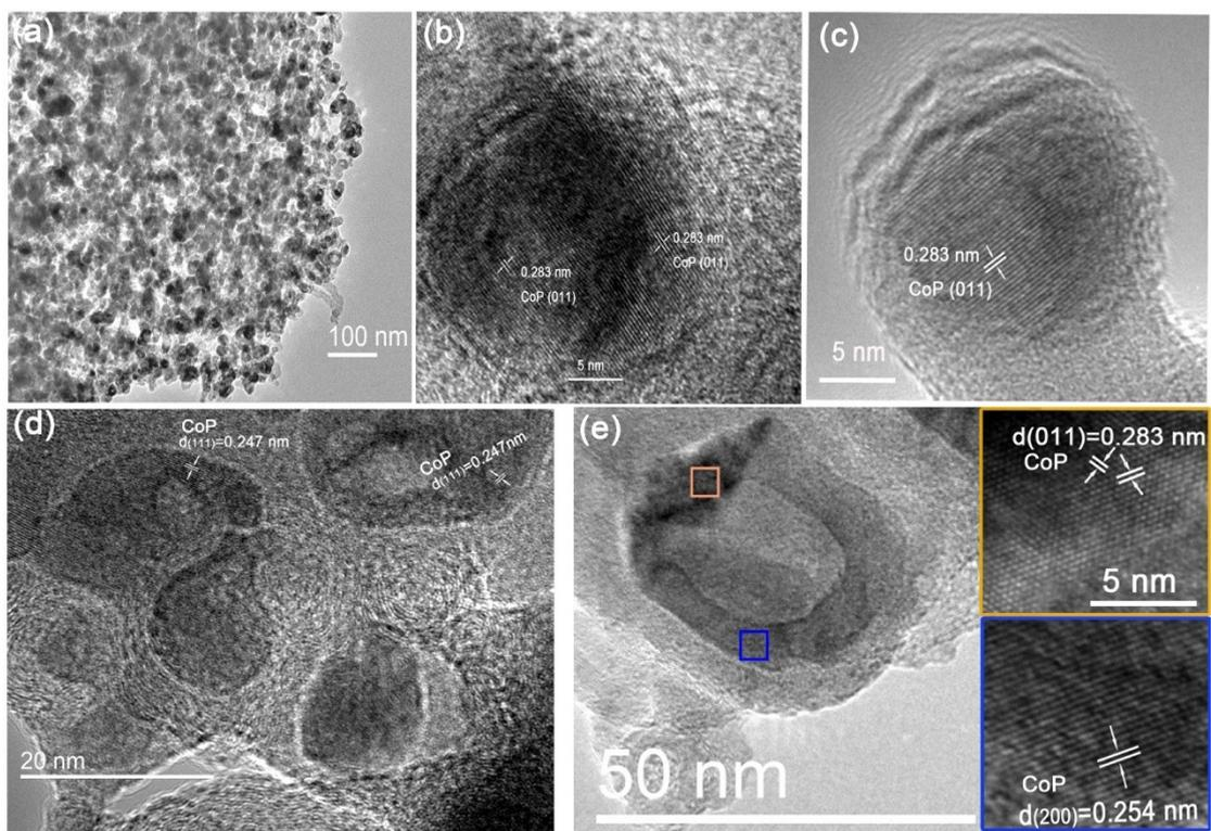
**Fig. S7** TEM images of the CoP-CNT/Ni<sub>2</sub>P/NF: (a) CoP-CNT nanosheet, (b) CoP NPs surrounded by CNTs in the nanosheet, (c) CoP NPs encapsulated by carbon layer. (d) and (e) some irregular hollow CoP NPs in the nanosheet.
