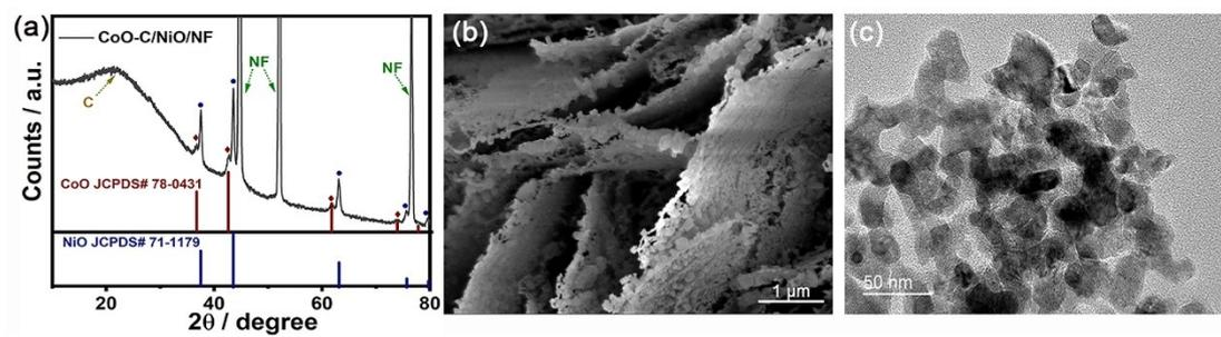
**Fig. S5** XRD pattern (a), SEM image (b) and TEM image (b) of the  $\text{Co}_2(\text{OH})_2(\text{BDC})$  nanosheet after calcination at 400 °C in pure Ar atmosphere.
