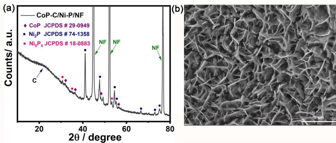
Fig. S18 XRD pattern (a) and SEM image (b) of the CoP-C/Ni-P/NF.
