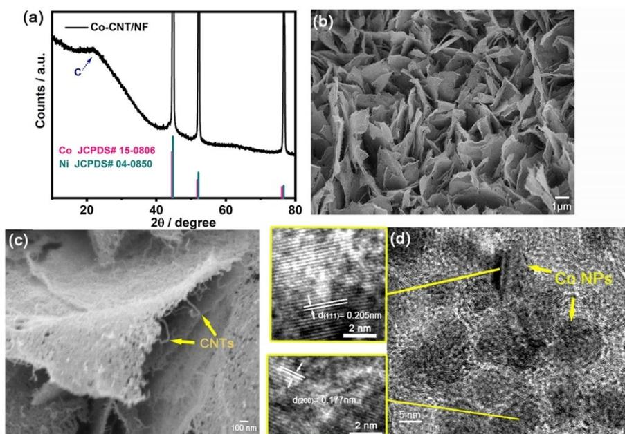
**Fig. S3** Characterization of the Co-CNT/NF: (a) XRD spectrum, (b) and (c) SEM images in different magnifications, (d) TEM image of Co-CNT nanosheet. Inset: lattice fringes of Co nanoparticles.
