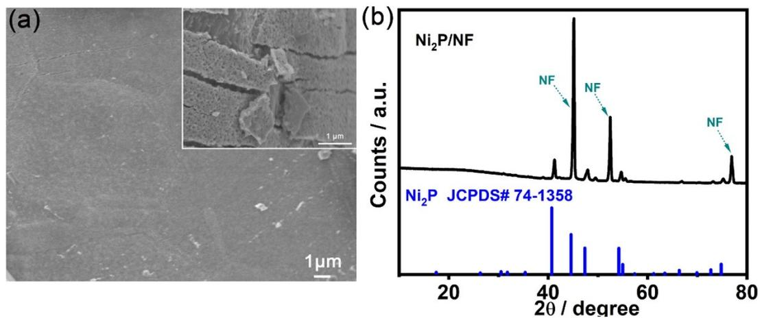
**Fig. S12** (a) Low and high magnification (Inset) SEM image of Ni<sub>2</sub>P/NF, (b) XRD pattern of Ni<sub>2</sub>P/NF.
