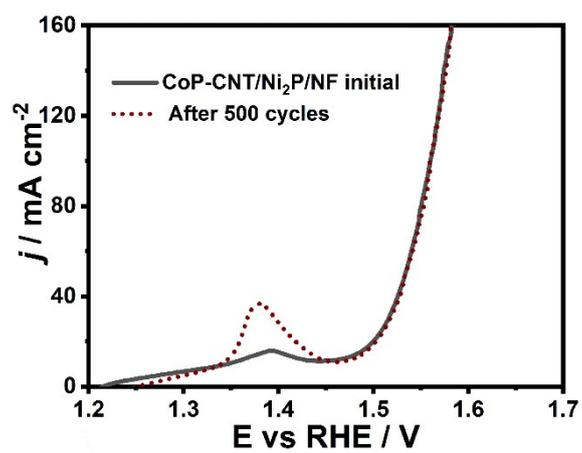
**Fig. S21** The LSV curve of the CoP-CNT/Ni<sub>2</sub>P/NF towards OER in 1.0 M KOH before and after 500 cycles.
