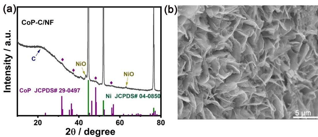
**Fig. S19** XRD pattern (a) and SEM image (b) CoP-C/NF.
