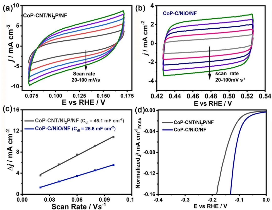
**Fig. S13** Cyclic voltammetry curves of the CoP-CNT/Ni<sub>2</sub>P/NF (a) and CoP-C/NiO/NF (b) at different scan rates from 20 mV s<sup>-1</sup> to 100 mV s<sup>-1</sup> in 1.0 M KOH solution. (c) The corresponding  $C_{dl}$  plots. (d) ECSA-normalized polarization curves of the CoP-CNT/Ni<sub>2</sub>P/NF and CoP-C/NiO/NF.
