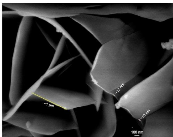
**Fig. S2** The enlarged SEM image of Co<sub>2</sub>(OH)<sub>2</sub>(BDC) nanosheet on the NiO/NF
