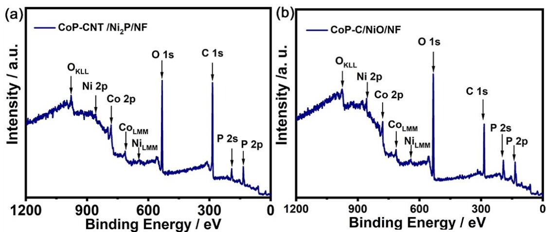
**Fig. S11** XPS survey spectra of the CoP-CNT/Ni<sub>2</sub>P/NF (a) and CoP-C/NiO/NF (b).
