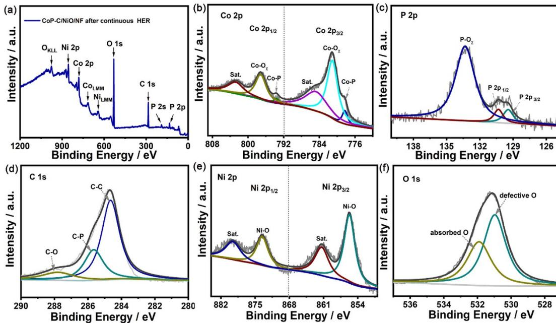
**Fig. S16** The XPS spectrum of the CoP-C/NiO/NF catalyst after 20 h electrolysis toward HER in 1.0 M KOH solution: (a) survey -scan spectra (b) Co 2p (c) P 2p (d) C 1s (e) Ni 2p (f) O 1s.
