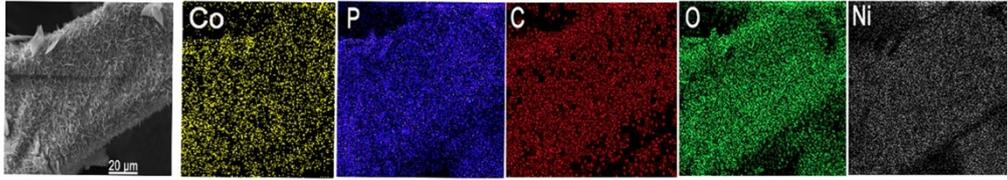
**Fig. S10** The energy-dispersive X-ray spectroscopy elemental mapping images of CoP-C/NiO/NF.
