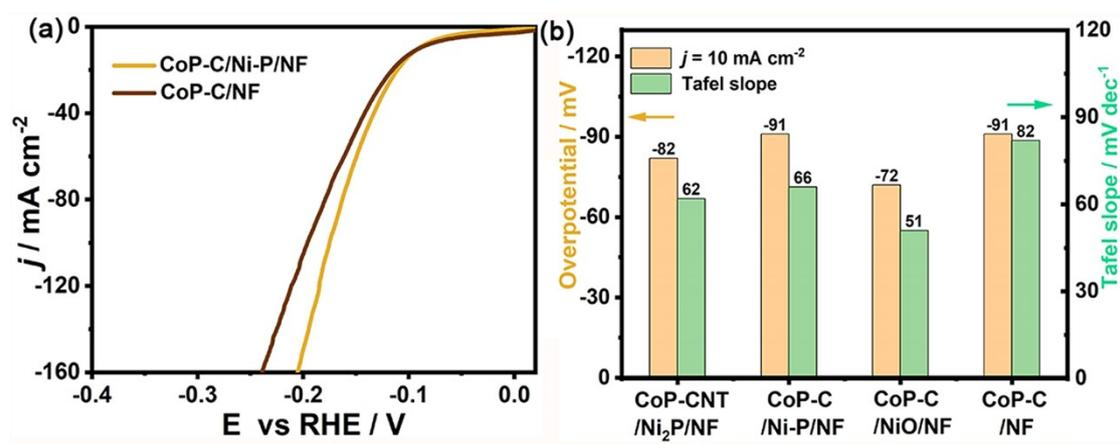
**Fig. S20** (a) polarization curves of the CoP-C/Ni-P/NF and CoP-C/NF toward HER in 1.0 M KOH solution at a scan rate of 5 mV s<sup>-1</sup>. (b) The histogram of the overpotential at  $j = 10$  mA cm<sup>-2</sup> and corresponding Tafel slope for the synthesized Co-based catalysts toward HER in 1.0 M KOH solution.
