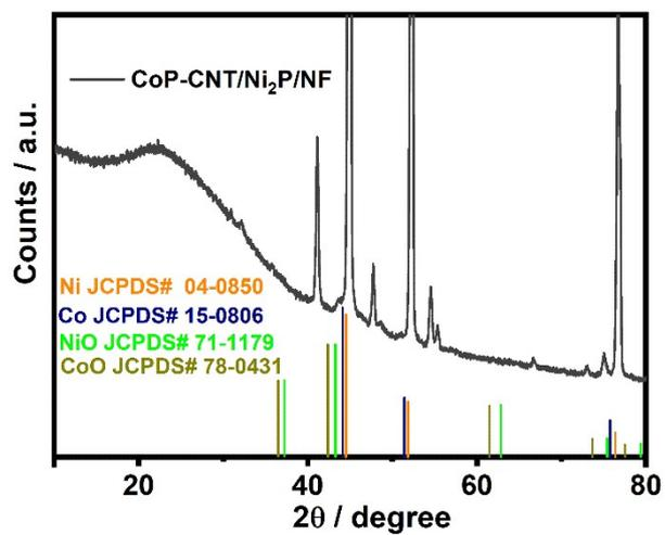
**Fig. S6** The spectrum to contrast the XRD pattern of CoP-CNT/Ni<sub>2</sub>P/NF and the standard card of metallic Co/Ni and CoO/NiO.
