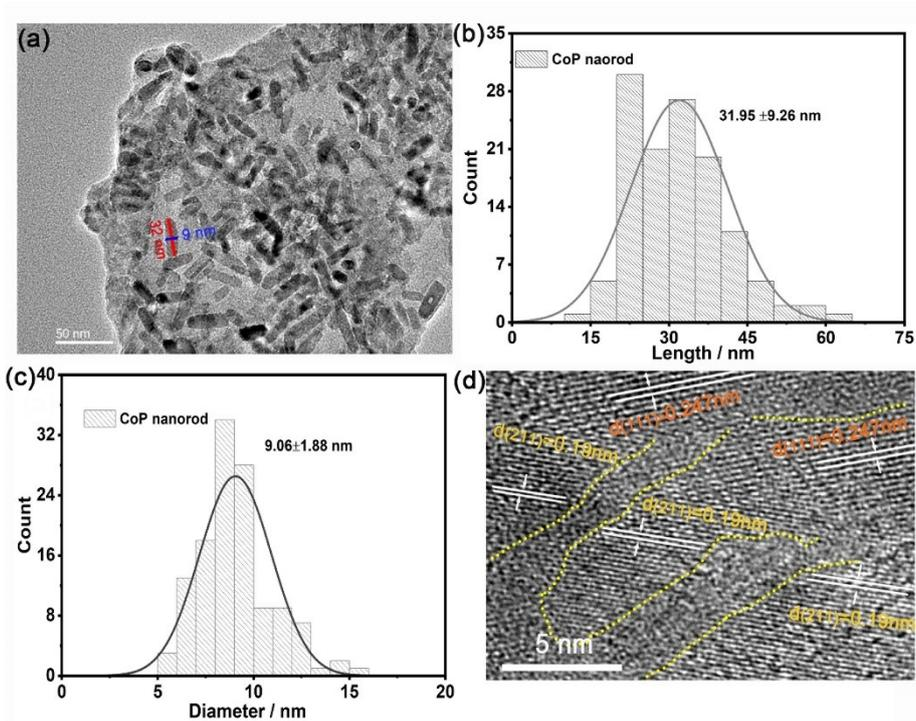
**Fig. S9** (a)TEM image of the CoP-C nanosheet in the CoP-C/NiO/NF. (b) and (c) the size distribution of the CoP nanorod. (d) HRTEM image of the CoP-C nanosheet in the CoP-C/NiO/NF (edge site)
