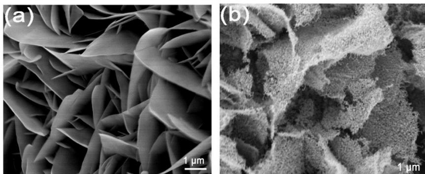
**Fig. S4** SEM images of the  $\text{Co}_2(\text{OH})_2(\text{BDC})/\text{NiO}/\text{NF}$  after calcination at 350 °C (a) and 450 °C (b) under 5%  $\text{H}_2$ -95% Ar mixed atmosphere for 1.5 h.
