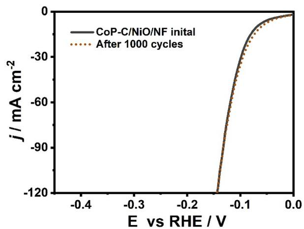
**Fig. S14** The LSV curve of the CoP-C/NiO/NF toward HER in 1.0 M KOH solution before and after 1000 cycles.
