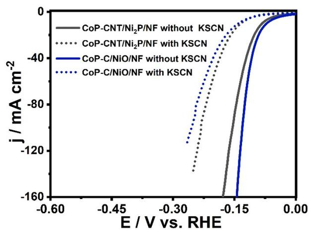
**Fig. S17** Polarization curves of the CoP-CNT/Ni<sub>2</sub>P/NF and CoP-C/NiO/NF with and without the addition of 10 mmol KSCN toward HER in 1.0 M KOH.
