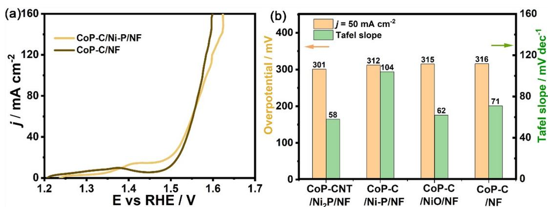
**Fig. S24** (a) Polarization curves of the CoP-C/Ni-P and CoP-C/NF towards OER in 1.0 M KOH at a scan rate of  $1\text{ mV s}^{-1}$ . (b) The histogram of the overpotential at  $50\text{ mA cm}^{-2}$  and corresponding Tafel slope for the synthesized Co-based catalysts towards OER in 1.0 M KOH.
