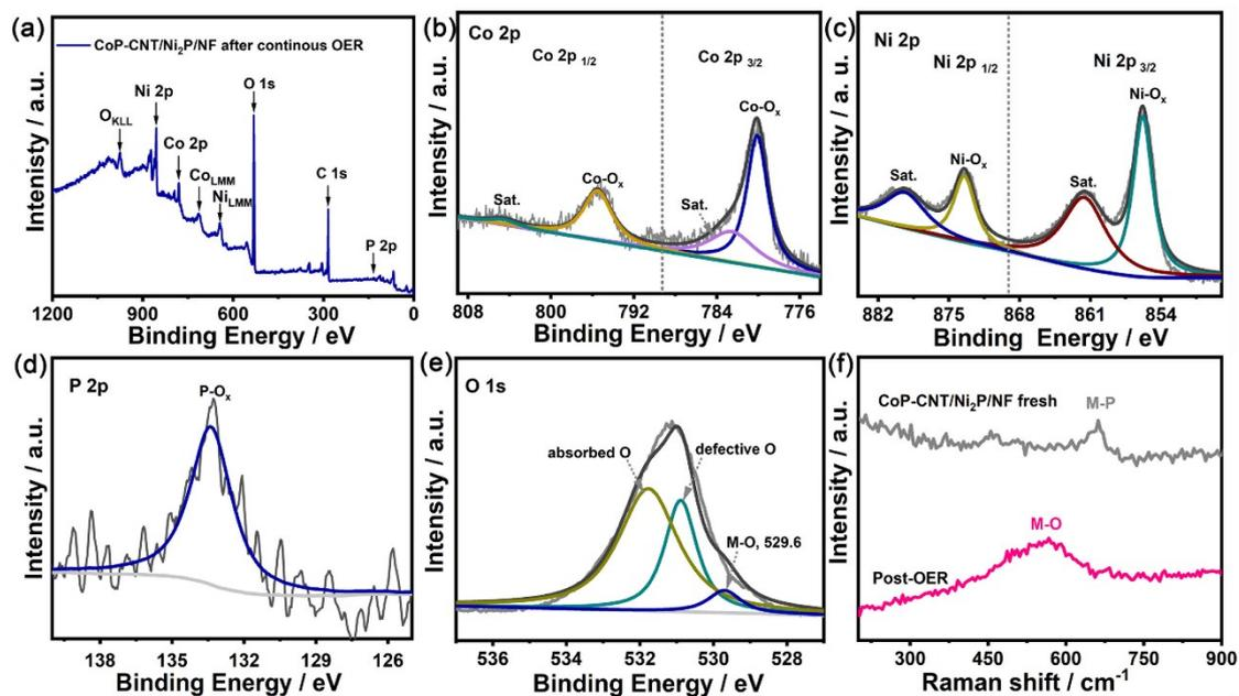
**Fig. S23** (a-e) The XPS spectrum of the CoP-CNT/Ni<sub>2</sub>P/NF catalyst after long-time electrolysis towards OER in 1.0 M KOH. (f) Raman spectra of the CoP-CNT/Ni<sub>2</sub>P/NF before and post OER.
