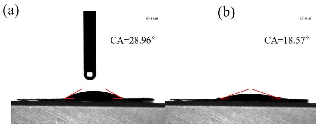
**Figure S6.** The water contact angle images of MOF 1 at first contact (a) and spread out (b).
