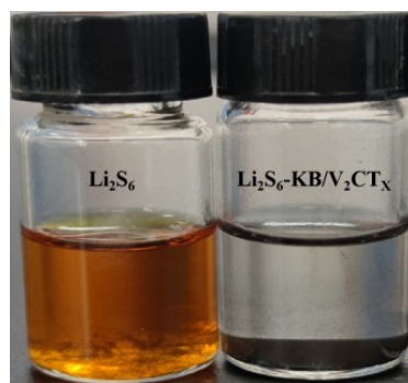
Fig. S4. Digital photographs of \text{Li}_2\text{S}_6 solution and after the addition of \text{KB/V}_2\text{CT}_x .
