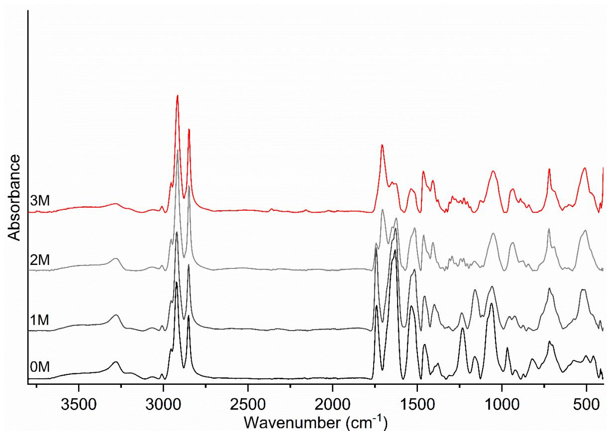
**Fig. S14** FTIR spectra (region 4000-500 cm<sup>-1</sup>) of the naturally aged model mixture: cinnabar and egg yolk after 0 month (0M) 1 month (1M), 2 month (2M) and 3 month (3M).
