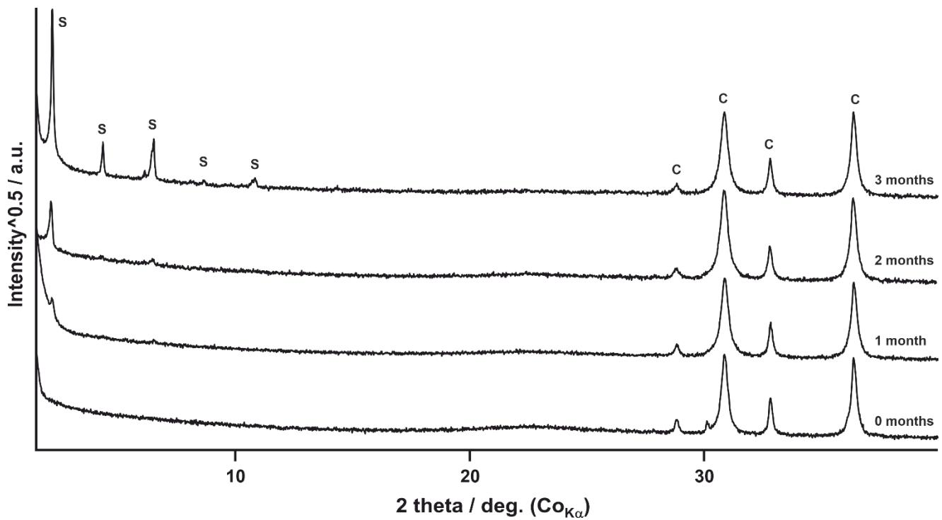
**Fig. S13** Full range XRPD patterns of the naturally aged model mixture: cinnabar and egg yolk after 0 ,1, 2 and 3 months.
