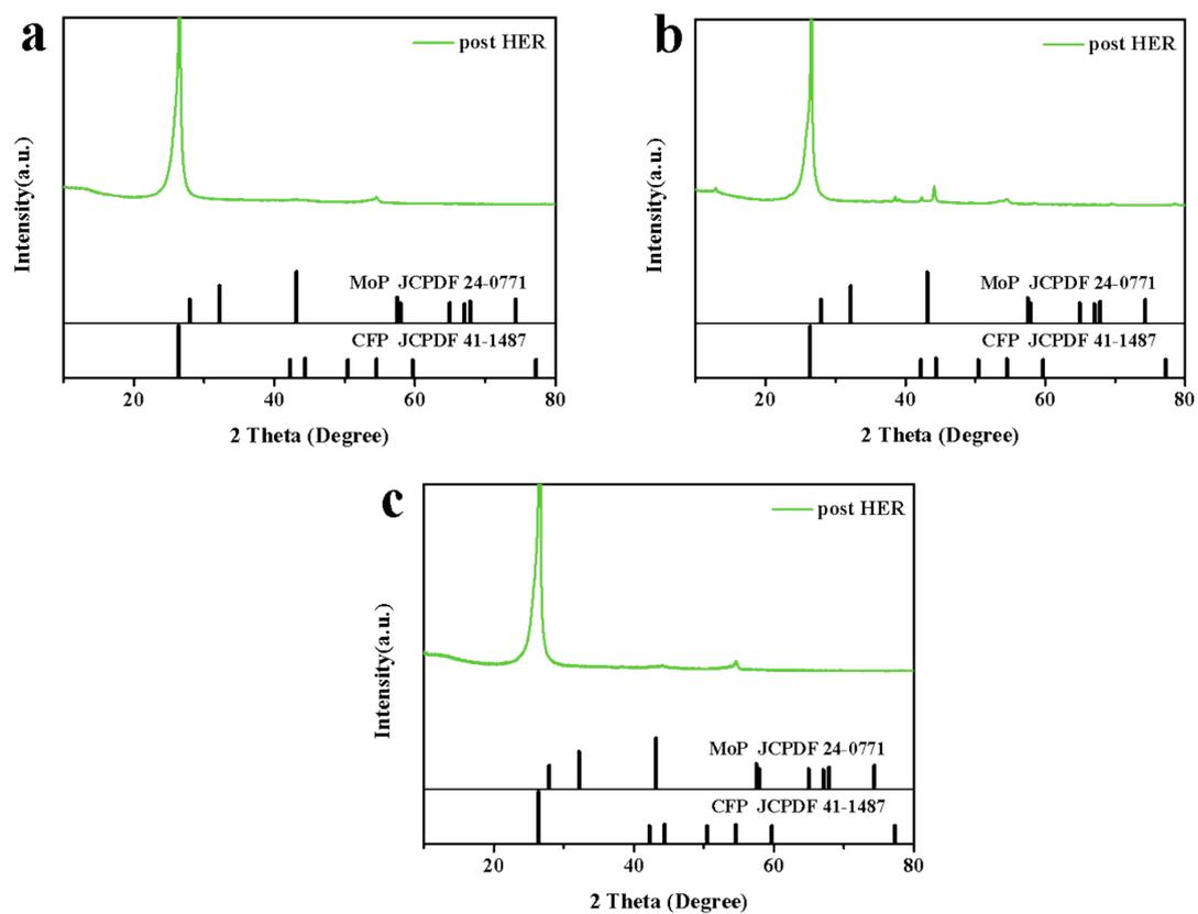
**Fig. S5.** XRD patterns of the Ru-MoP NWAs/CFP catalyst after HER durability tests in (a) 0.5 M H<sub>2</sub>SO<sub>4</sub>, (b) 1 M PBS, and (c) 1 M KOH.
