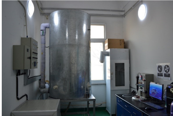
Figure S2. Picture of the isothermal cloud chamber (1 m 3 ).
