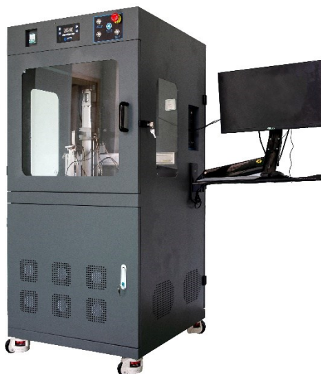
Supplementary Fig. 13 The Optical image of an ultrasonic battery scanner.
