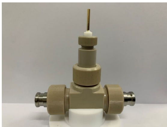
Fig. S17 Photograph of the home-made three-electrode cell.
