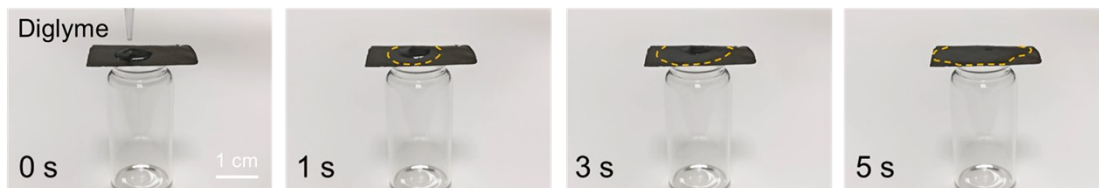
Figure S7. The wettability testing of L700 with diglyme, where the 100 \mu L diglyme can be fully absorbed in a piece of L700 since no diglyme can penetrate the L700.
