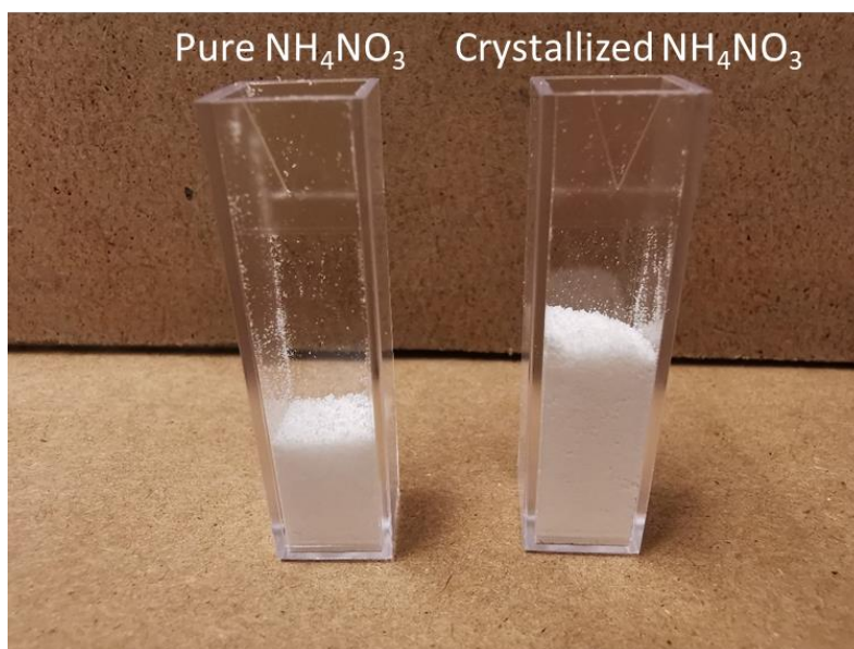
Figure S6. The volume of pure \text{NH}_4\text{NO}_3 salt and crystallized \text{NH}_4\text{NO}_3 (with and 0.5% SVBS) with the same weight of 1 g.
