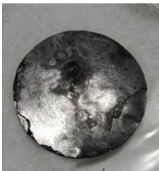
Fig. S16 A 200 \mu\text{m} GN3 pressed film, showing a shiny surface, indicative of high conductivity.
