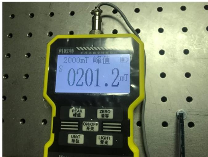
**Figure S6.** The magnetic induction field strength is measured by a Tesla meter.
