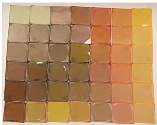
149 Fig. S1 (A) Photograph of the perovskite films (No.8-No.49) annealed at 170 °C for 10 min 150 arranged in the same order as in the composition matrix of Fig. 1A. (B) The different colors of 151 CsPbI 3 films annealed at different temperatures.
