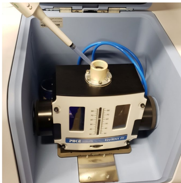
Figure S. 1 Experimental setup for FTIR measurements using a PikeVeeMax II ATR accessory and a 60^\circ face-angled Ge crystal. The known amounts of \text{NaHCO}_3 or \text{Na}_2\text{CO}_3 are added to \text{CH}_3\text{OH} contained in the Jackfish cell.
