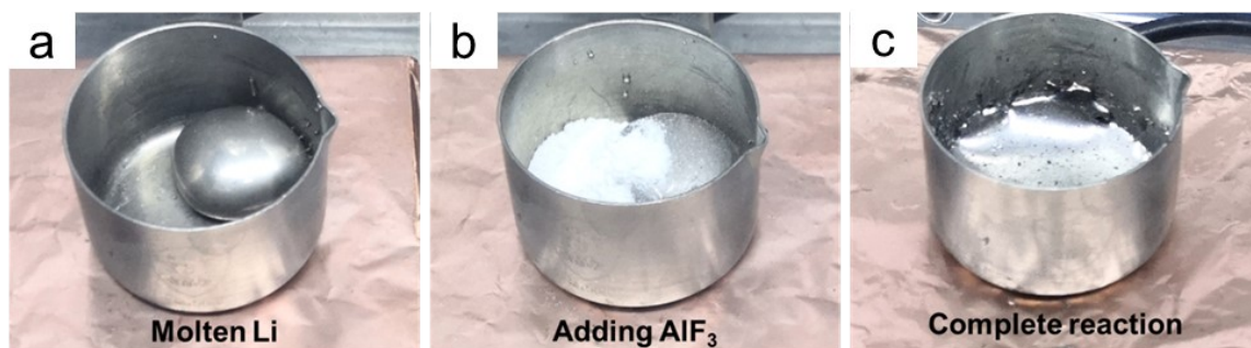
Figure S3. The fabrication process of adding AlF 3 into molten Li under stirring at 300 °C. AlF 3 experienced conversion and alloying reactions upon the reaction with molten Li, generating LiF, Li 9 Al 4 with excessive Li.
