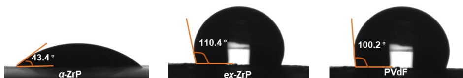
Fig. S8 Contact angle measurements of water on \alpha -ZrP, ex -ZrP and PVdF.
