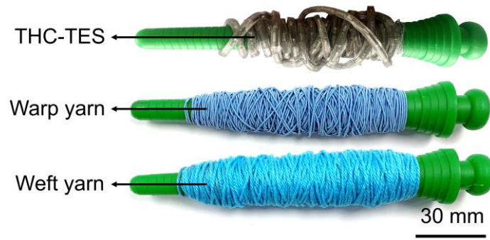
Supplementary Figure 12 | Optical images of THC-TES, warp yarn (elastic) and weft yarn using in TET.
