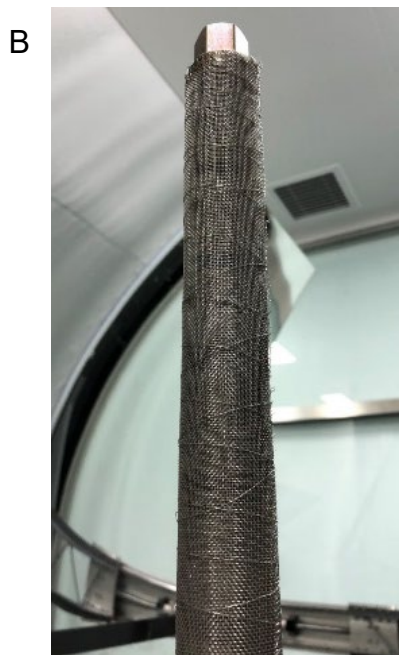
Fig. S8. Sequential separation-driven SMR reactor for integration with parabolic trough solar collector. (A) The Pd-Ag membrane tube wrapped by a stainless-steel mesh. (B) The Pd-Ag membrane tube with a stainless-steel mesh housing six sets of Ni/MgO-Al 2 O 3 catalyst and hydrotalcite CO 2 sorbent combination.
