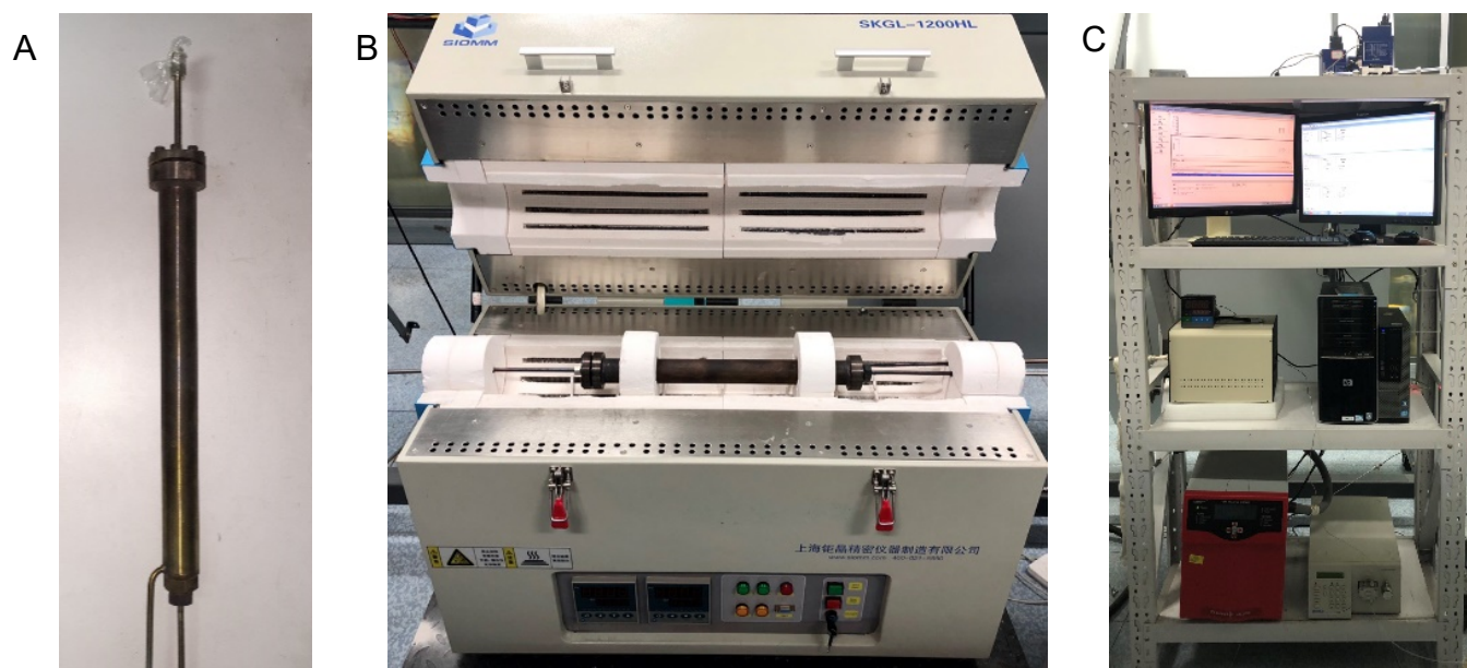
Fig. S12. Experimental platform for proof-of-concept studies of sequential separation-driven SMR. (A) The reactor corresponding to Fig. 1 of the main text. (B) The reactor mounted in an electric furnace for measurements. (C) Online measurement and analysis system.
