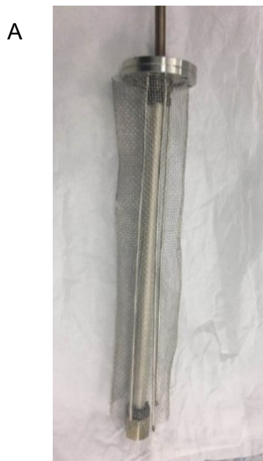
Fig. S8. Sequential separation-driven SMR reactor for integration with parabolic trough solar collector. (A) The Pd-Ag membrane tube wrapped by a stainless-steel mesh. (B) The Pd-Ag membrane tube with a stainless-steel mesh housing six sets of Ni/MgO-Al 2 O 3 catalyst and hydrotalcite CO 2 sorbent combination.
