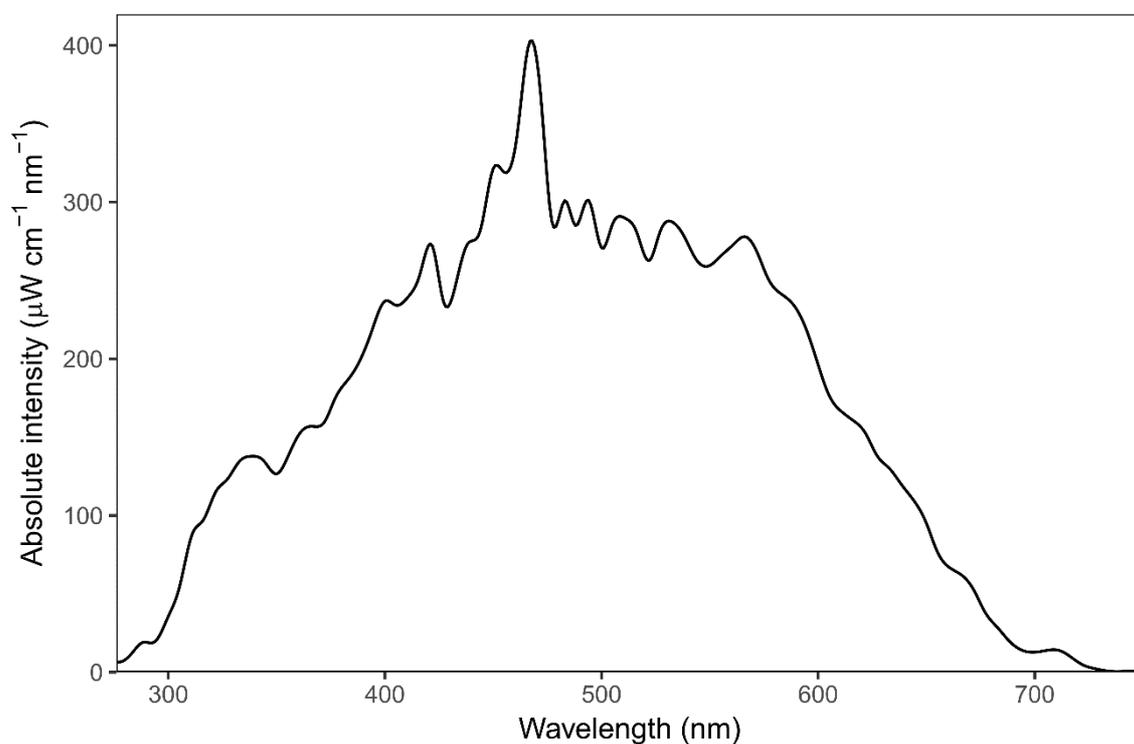
Fig. S4. Absolute light intensity as a function of the wavelength for the Xenon Arc Lamp as measured in the quartz tube after the liquid light guide. The light spectrum was characterized with a calibrated spectroradiometer ILT 900C (International Light®) at a wavelength resolution of 1 nm. Significant irradiation ( $I(\lambda) > 0.1 \times I_{\text{mean}}$ ) ranged from [270;720] nm.
