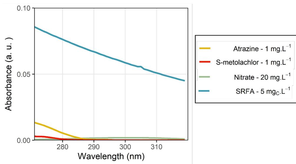
Fig. S3 UV-vis absorption spectra of atrazine, *S*-metolachlor, nitrates and SRFA at experimental concentrations. The absorption spectra for nitrates was extracted from Gaffney et al.<sup>5</sup>
