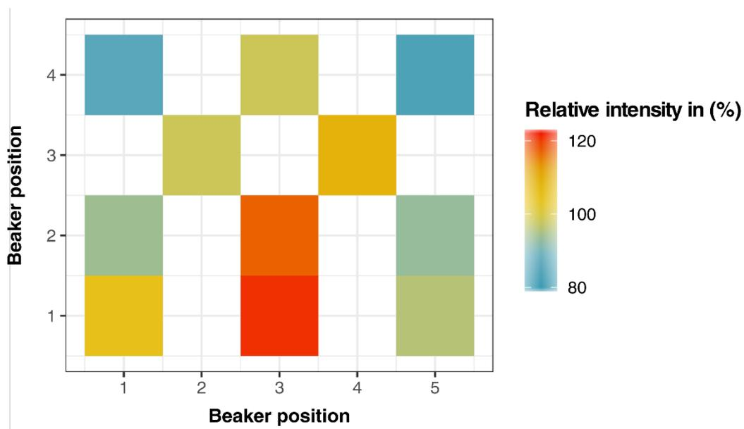
Fig. S2. Spatial distribution of irradiation intensity within the light-proof box. Transparent places correspond to empty spaces where the irradiation intensity was not measured within the light-proof box.
