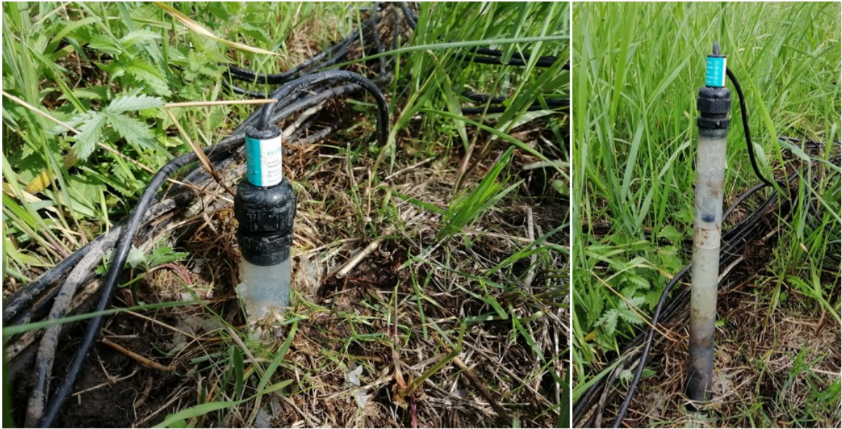
Figure S6 Image of a reference electrode installed at site Speicherkoog embedded within a salt bridge to close the electrical circuit with the soil. Please note, the salt bridge was removed from the soil on the right image for maintenance.
