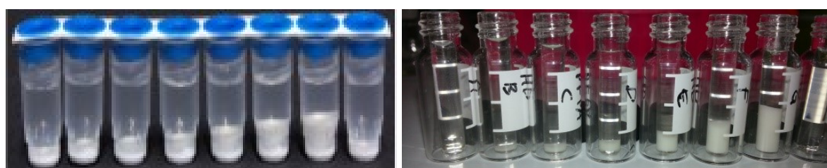
Figure S2. A 6 vial sorbent-dilution series strip from the TRANSIL XL 96-well plate system transferred to glass inserts.
