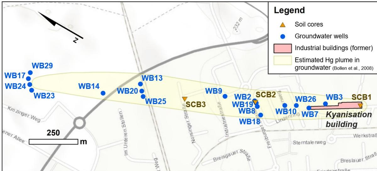
*Figure S1.2: Map of **site B** showing groundwater well and soil core sampling locations as well as the former industrial buildings. Map produced in ArcGIS (ESRI). The estimated groundwater plume is taken from Bollen et al. (2008).*
