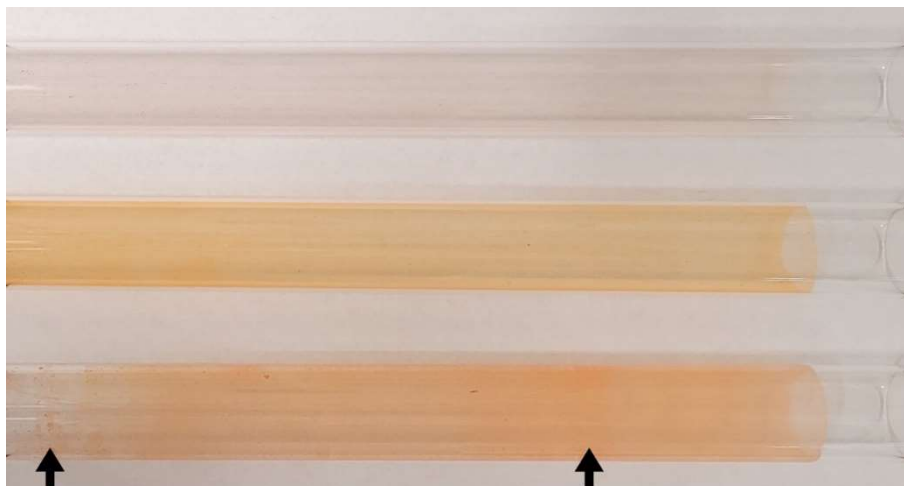
Fig. S1. Representative substrate tubes with thin films of sunset yellow, showing a sample prepared by rolling with dye solution, exhibiting bands and patches indicated with arrow (bottom); a sample prepared by atomizing and depositing particles, before (middle) and after (top) deliquescence and removal of water. Before deliquescence, the sample is uniform but coarse and opaque; afterwards, it is uniform, smooth, and translucent.
