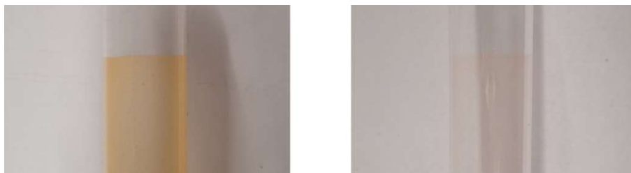
Fig. S2. Representative substrate tubes with thin films of sunset yellow, after deliquescence (left) and after drying (right). Upon deliquescence, the sample increases in opacity significantly; after drying, it decreases in opacity, to be much more translucent than the initial tubes before deliquescence.
