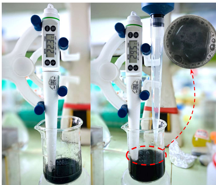
Figure S7. The temperature of sludge carbon-containing suspended slurry before and after adding HF
