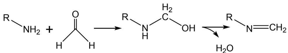
**Figure S4.** The mechanism of the free amino group reacts with formaldehyde.
