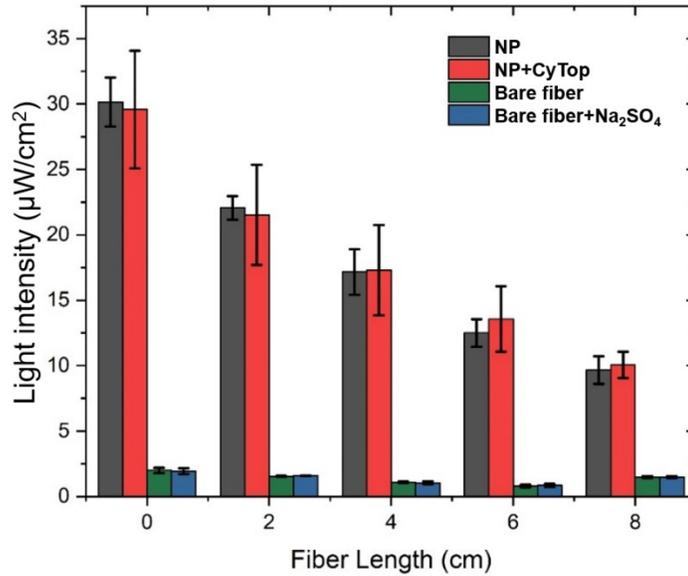
**Figure SI.5** Light irradiance measured at different distances along the optical fiber with 200 nm nanoparticles, 200 nm nanoparticles with CyTop™ polymer, without NP (bare fiber), and bare fiber with Na<sub>2</sub>SO<sub>4</sub>.
