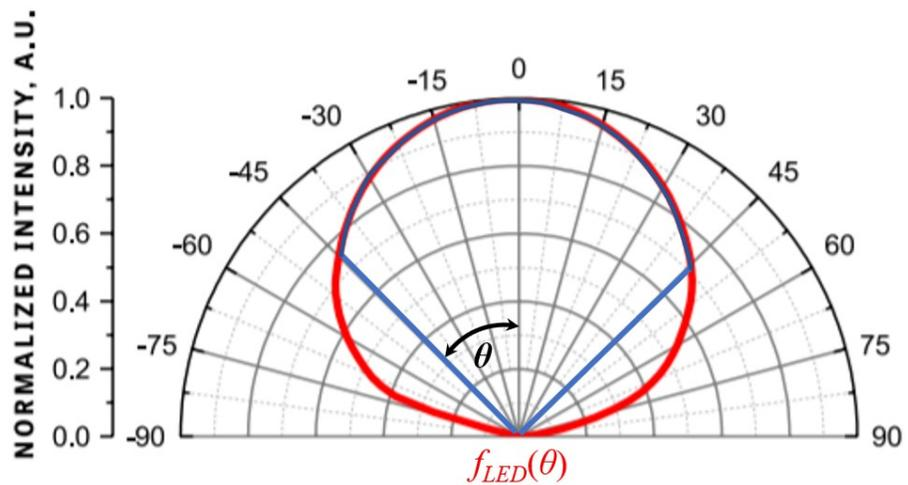
**Figure SI.8** Radiation pattern of UV-C LED in the first principle model.
