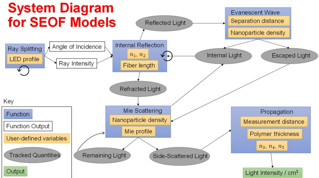
**Figure SI.6** System diagram of SEOF scattering efficiency model.
