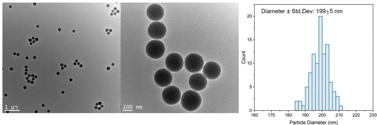
**Figure SI.4** TEM images and the size distribution of silica sphere nanoparticles.
