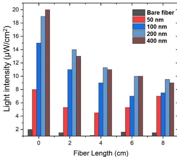
**Figure SI.2** Effect of nanoparticle size on 265 nm UV-C LED launched optical fibers.
