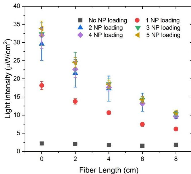
**Figure SI.3** Effect of nanoparticle loading on 265 nm UV-C LED launched optical fibers.
