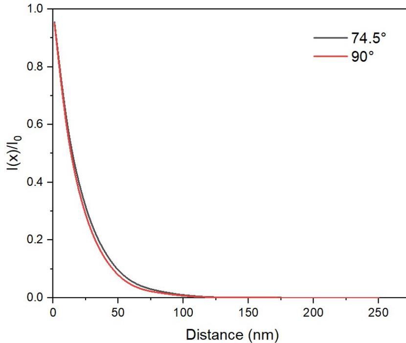
**Figure SI.9** Evanescent wave intensity as a function of radial distance (nm) from the optical fiber surface for 265 nm light at an incident angle of 90° and 74.5° (minimum).
