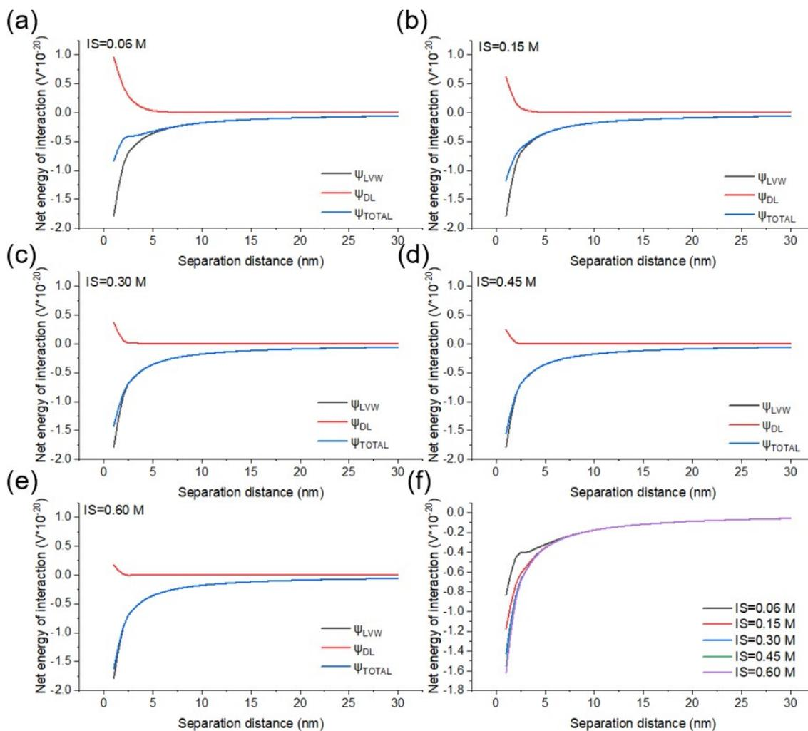
**Figure SI.11** Energy of interaction between two aminated silica nanoparticles with separation distance under ionic strength at (a) 0.06 M, (b) 0.15 M, (c) 0.30 M, (d) 0.45 M, and (e) 0.60 M. (f) shows the net energy of interaction under ionic strength from 0.06 M to 0.60 M.  $\Psi_{LVW}$ ,  $\Psi_{DL}$  and  $\Psi_{TOTAL}$  represents the potential for attraction by London van der Waals forces, potential for repulsion due to double layer repulsion and total energy barrier, respectively.
