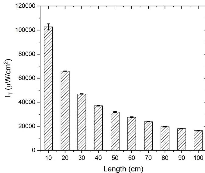
**Figure SI.1** UV-C light attenuation inside the high-OH Thorlabs optical fiber. The distance between fiber cut end and LED is zero.
