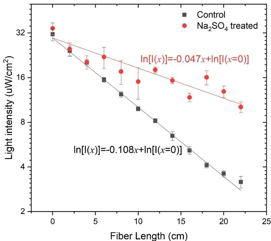
**Figure SI.12** Natural logarithm fit of light intensity along optical fiber with and without different concentration of ionic strength treatment. Slope of fitted equation represents the scattering coefficient ( $\alpha$ ) at each condition.
