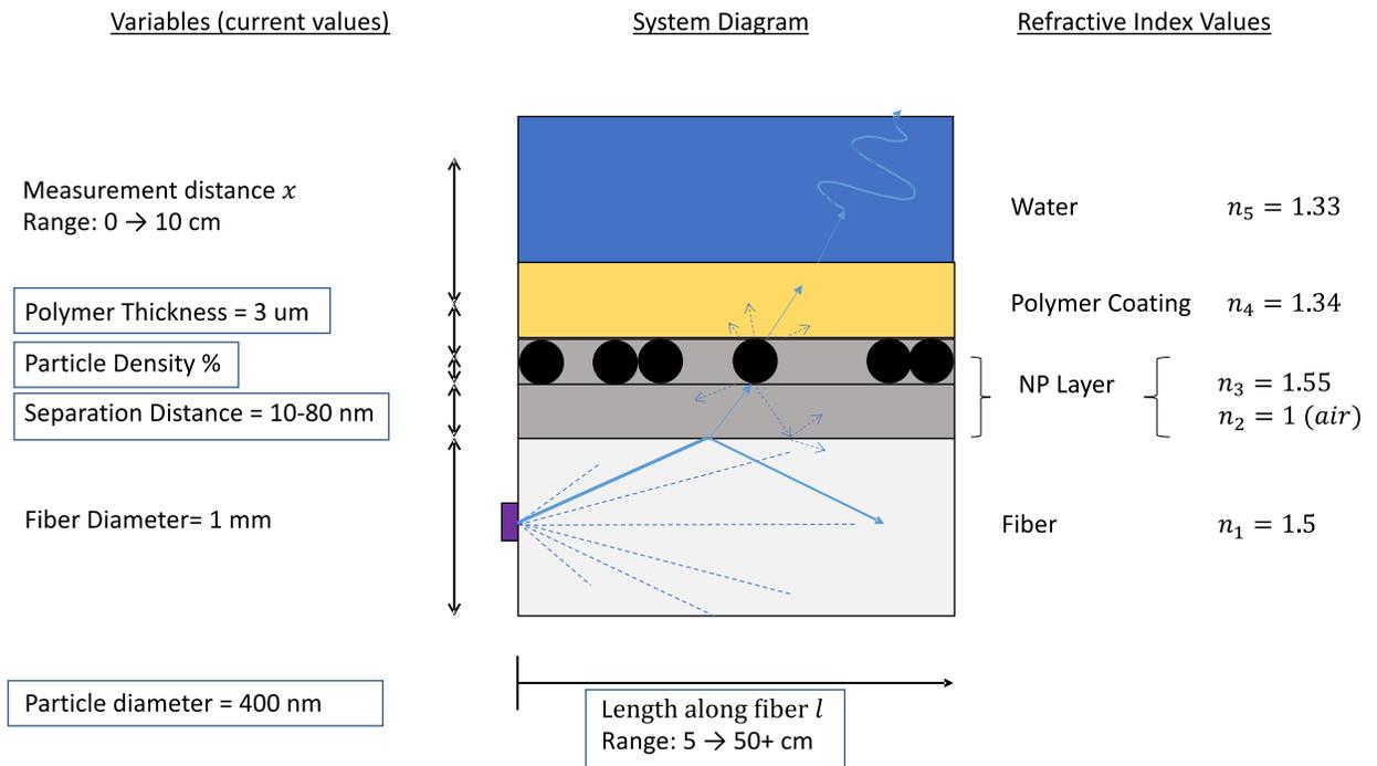
**Figure SI.7** Scattering efficiency model variables and input parameters.
