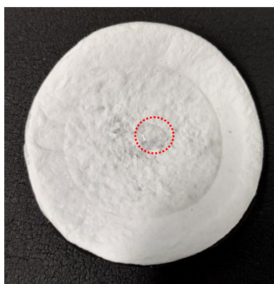
Fig. S8 Digital photo of the large water droplets collected on the hydrophobic MHCH&SiO 2 side of Janus membrane.
