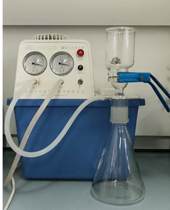
Fig. S1 Digital photo of the filter facility and the vacuum pump.
