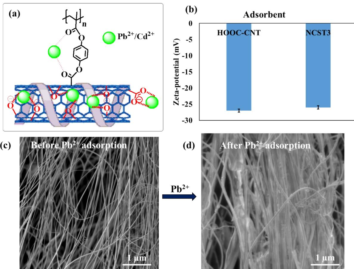
**Figure S4.** (a) Schematic illustration of proposed interactions between NCST3 adsorbent and HMIs, (b) Zeta potential of HOOC-CNT and NCST3 adsorbent, and (c) SEM image of NCST3 adsorbent before Pb<sup>2+</sup> adsorption, and (d) SEM image of NCST3 adsorbent after Pb<sup>2+</sup> adsorption.
