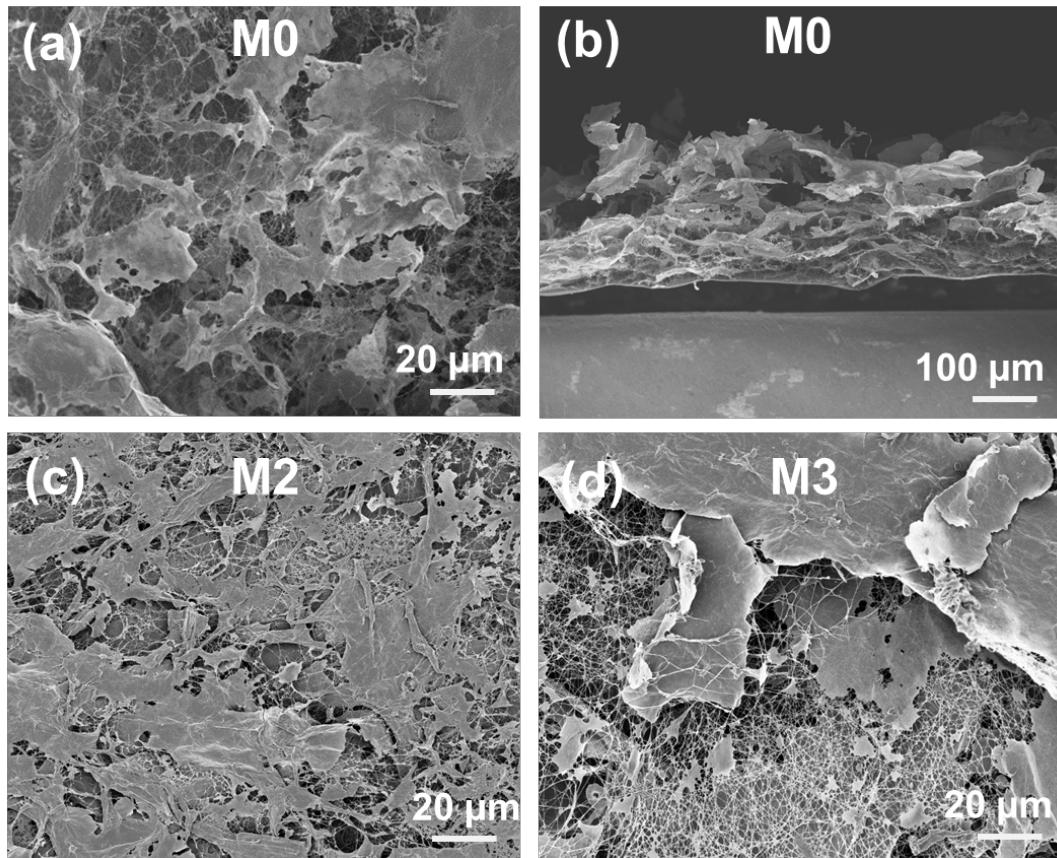
**Fig. S3.** SEM morphology of rGO/BNC membrane (a) top surface and (b) cross section, top surface morphology of rGO/BNC:BNC membranes (c) M2 and, (d) M3.
