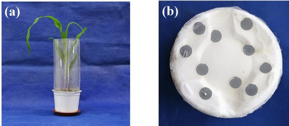
**Fig. S2.** Experimental culture pot design: the top (a) and bottom (b) of pot were covered with transparent plastic cylinders (height 20 cm) and nylon mesh (30  $\mu\text{m}$  pore diameter) for keeping from earthworm escaping.
