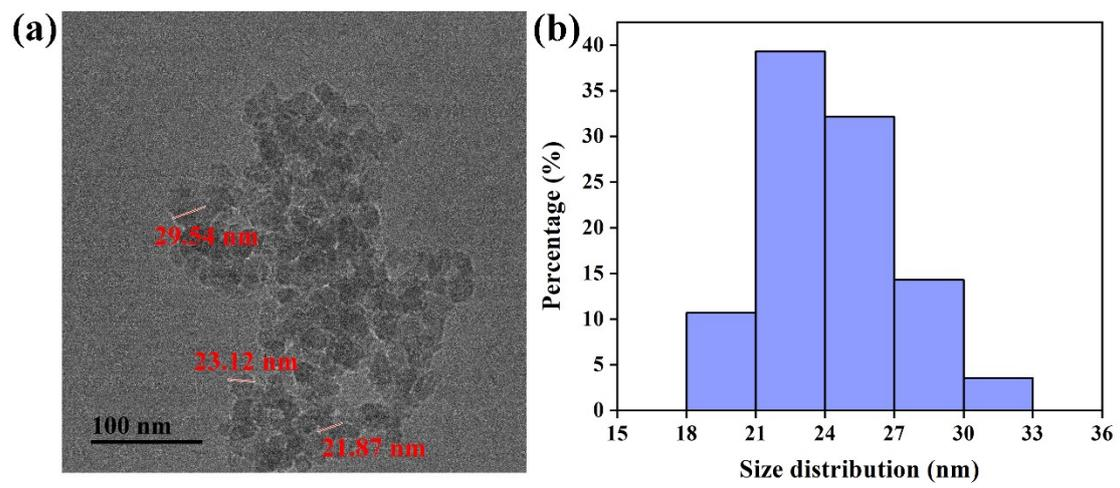
**Fig. S1.** TEM image (a) and size distribution (b) of SiO<sub>2</sub> NMs.
