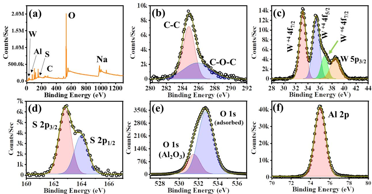
**Figure S3: Surface analysis of catalyst after five cycles. (a) XPS Survey scan. Individual high-resolution (b) C scan, (c) W scan, (d) S scan, (e) O scan and (f) Al scan.**
