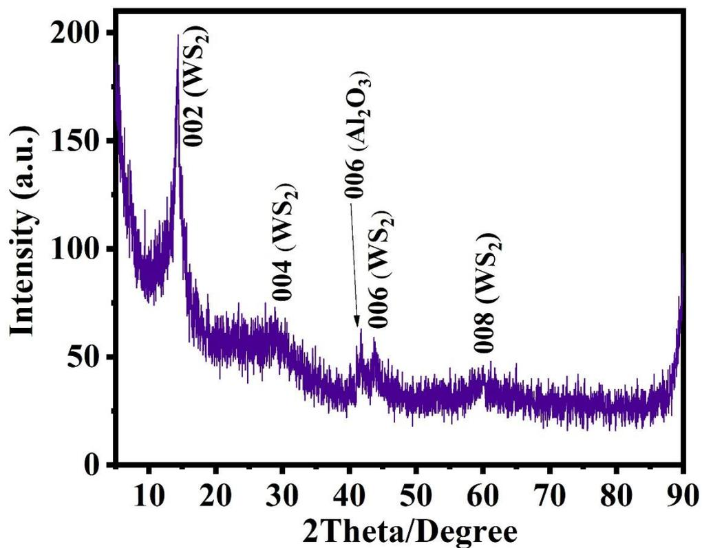
Figure S4: XRD analysis of WS<sub>2</sub> grown over sapphire substrate.
