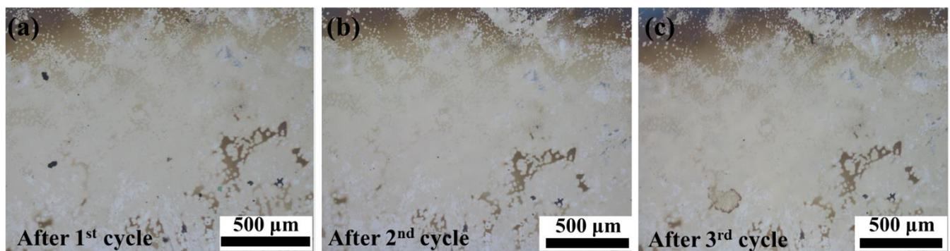
**Figure S2: Optical images shows recovery of catalyst after three piezocatalytic cycles.**
