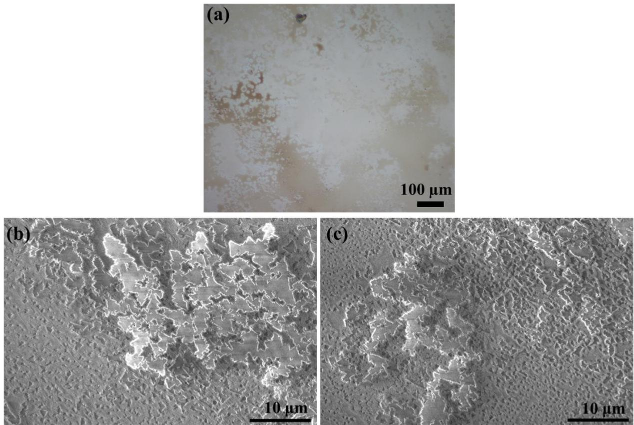
**Figure S1: (a) Optical image of large area growth of few layer WS<sub>2</sub> is shown. (b) and (c) FESEM image to show coalescence and multilayer formation.**
