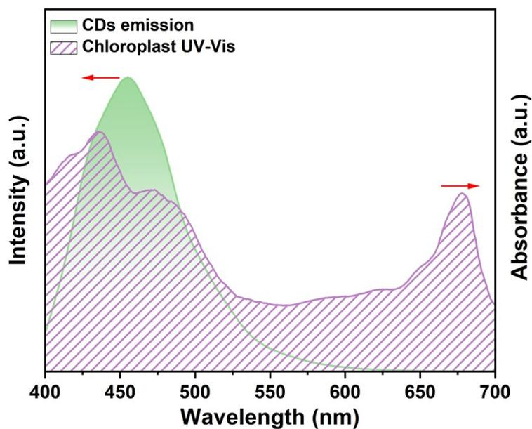
**Fig. S2** Emission spectrum of CDs excited at 360 nm and UV-Vis spectrum of chloroplasts isolated from the untreated lettuce leaves.
