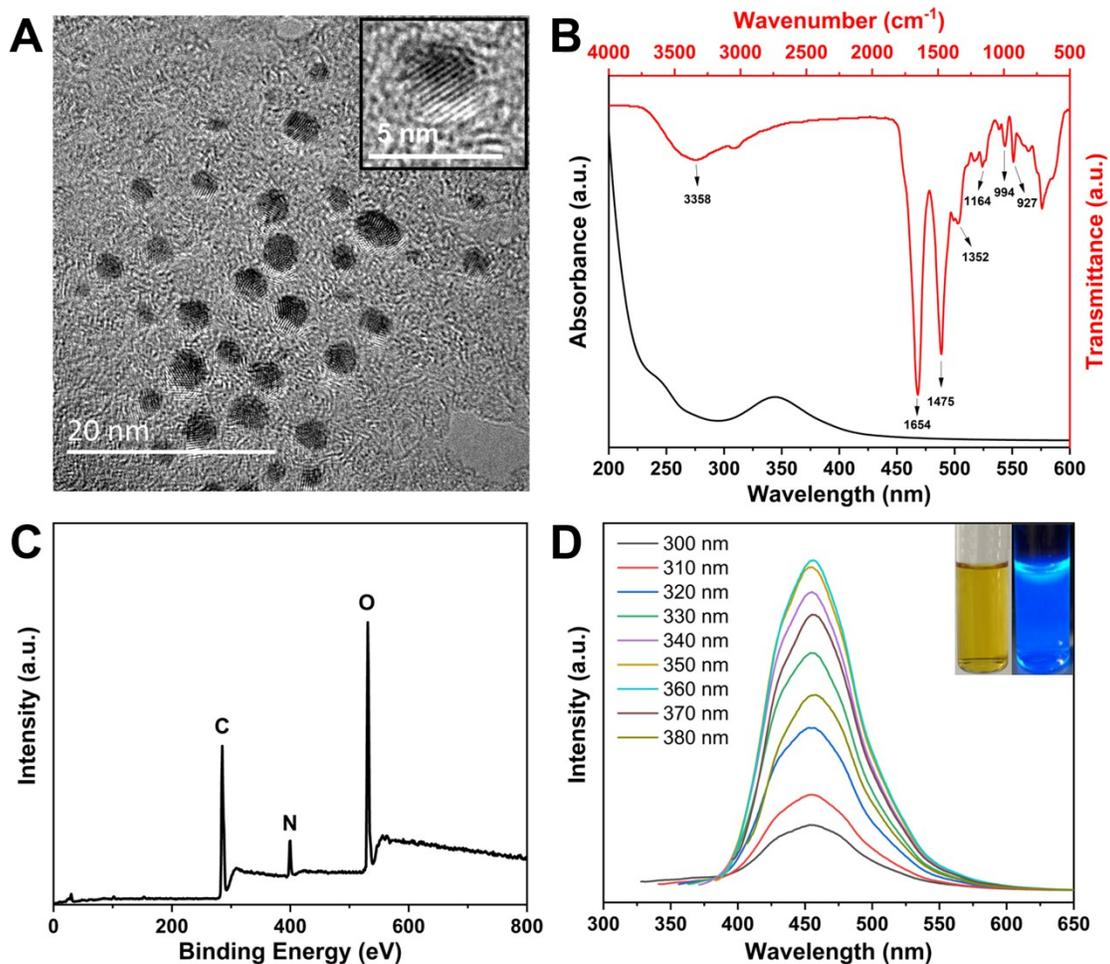
**Fig. S1** Characterization of CDs. (A) TEM image (inset: a high-resolution TEM image of single CDs particles). (B) FTIR and UV-Vis spectra of CDs. (C) Full XPS spectrum of CDs. (D) Emission spectra of CD recorded for progressively longer excitation wavelength of 10 nm increments from 300 to 380 nm (inset: the photograph of CDs under visible light and UV light at 370 nm, respectively).
