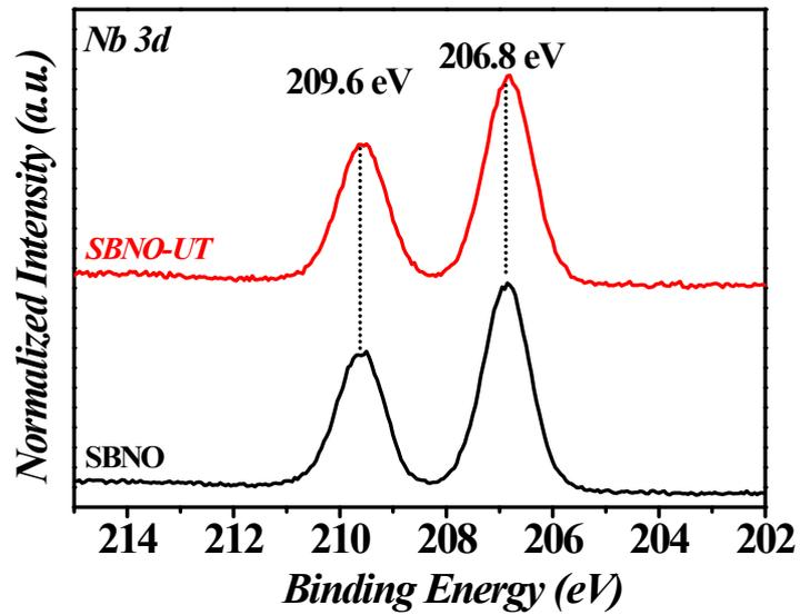
**Figure S7.** Comparative high resolution XPS spectra of Sr 3d and Nb 3d of SBNO and SBNO–UT, respectively.
