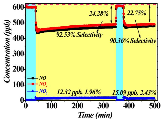
**Figure S12.** Long-term NO decomposition over defective SBNO-UT and light irradiation (NO in Ar).
