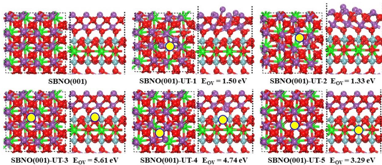
**Figure S5.** Calculated the structures and the vacancy formation energies of oxygen with assorted coordination environments on the SBNO (001) surface.
