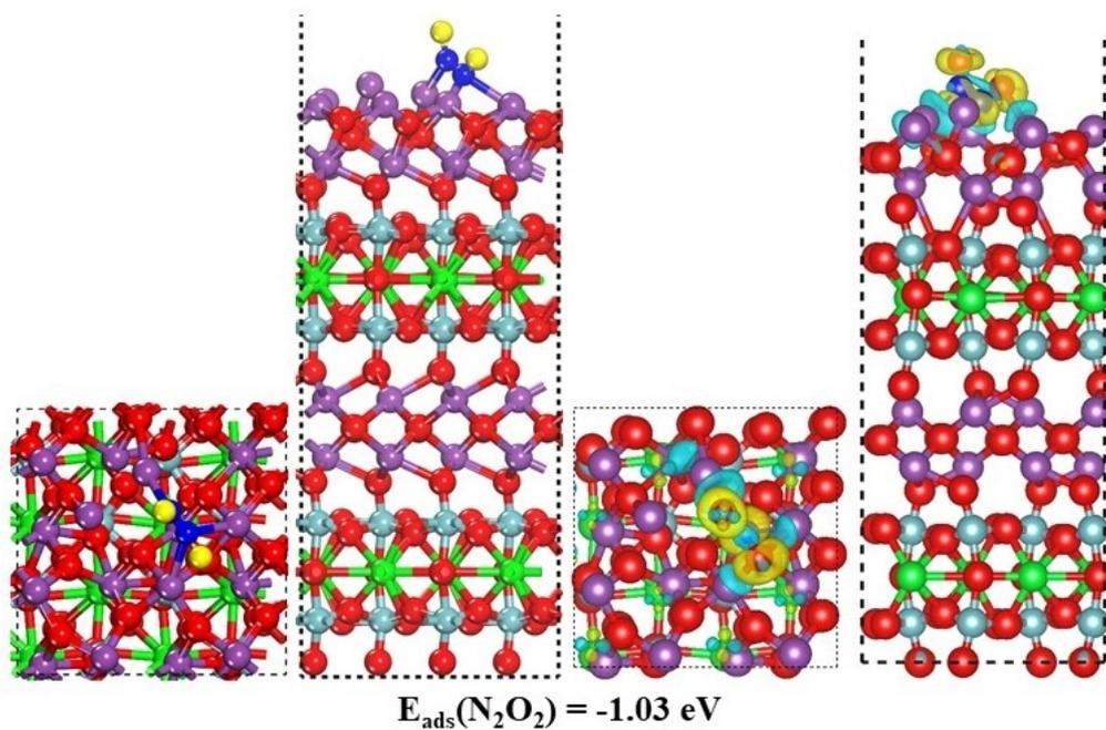
**Figure S11.** Calculated structures, spin-polarized charge densities and adsorption energies of two NO molecules adsorbed on SBNO–UT surface. Red: O atoms; green: Sr atoms; purple: Bi atoms; light blue: Nb atoms; Blue: N atoms, Yellow: O atoms in NO, respectively.
