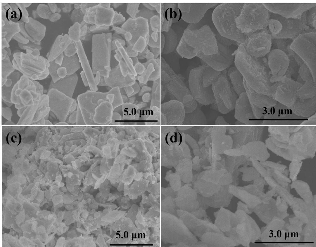
**Figure S4.** SEM images of SBNO samples prepared in HCl aqueous solution.
