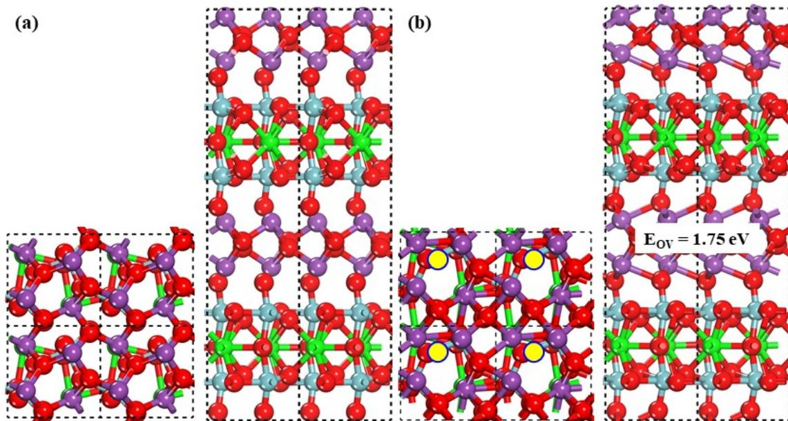
**Figure S6.** Calculated the structure and the vacancy formation energies of oxygen vacancies on the bulk of SBNO. (a) bulk of SBNO, (b) the oxygen vacancy of SBNO.
