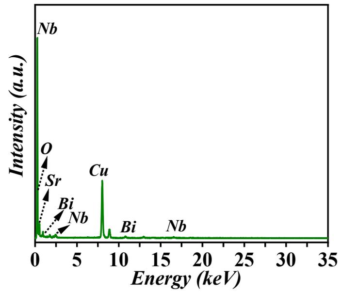
**Figure S3.** EDS spectra of SBNO–UT samples.
