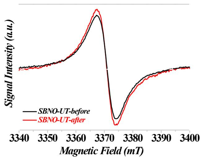
**Figure S13.** Comparative EPR spectra of SBNO-UT before and after the photocatalytic NO decomposition tests.
