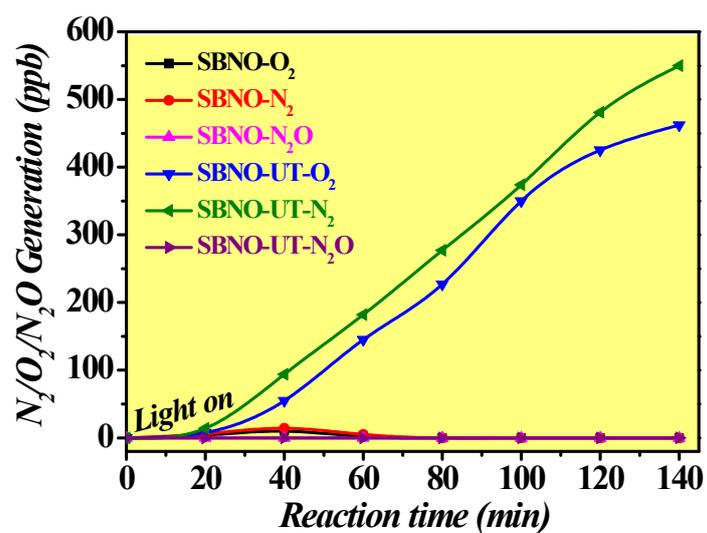
**Figure S10.** Formation of photocatalytic NO decomposition products with the assistance of SBNO and SBNO-UT, respectively.
