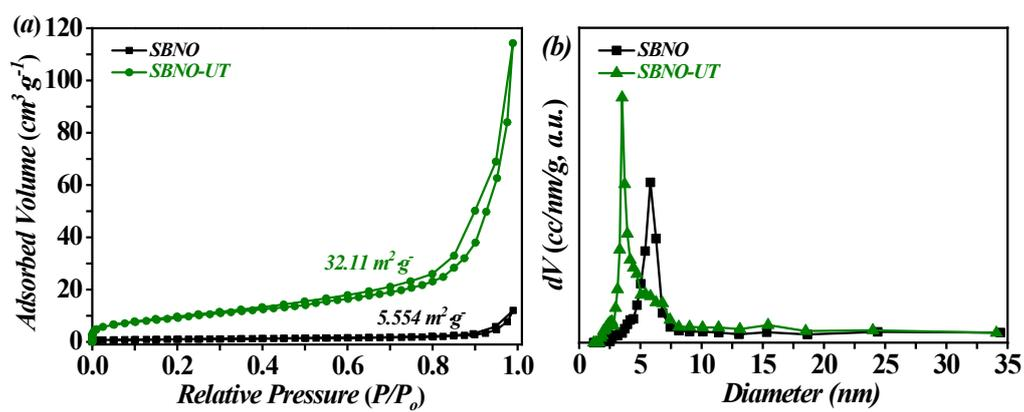
**Figure S9.** (a) Nitrogen adsorption-desorption isotherms, and (b) *pore size distribution* of SBNO and SBNO-UT, respectively.
