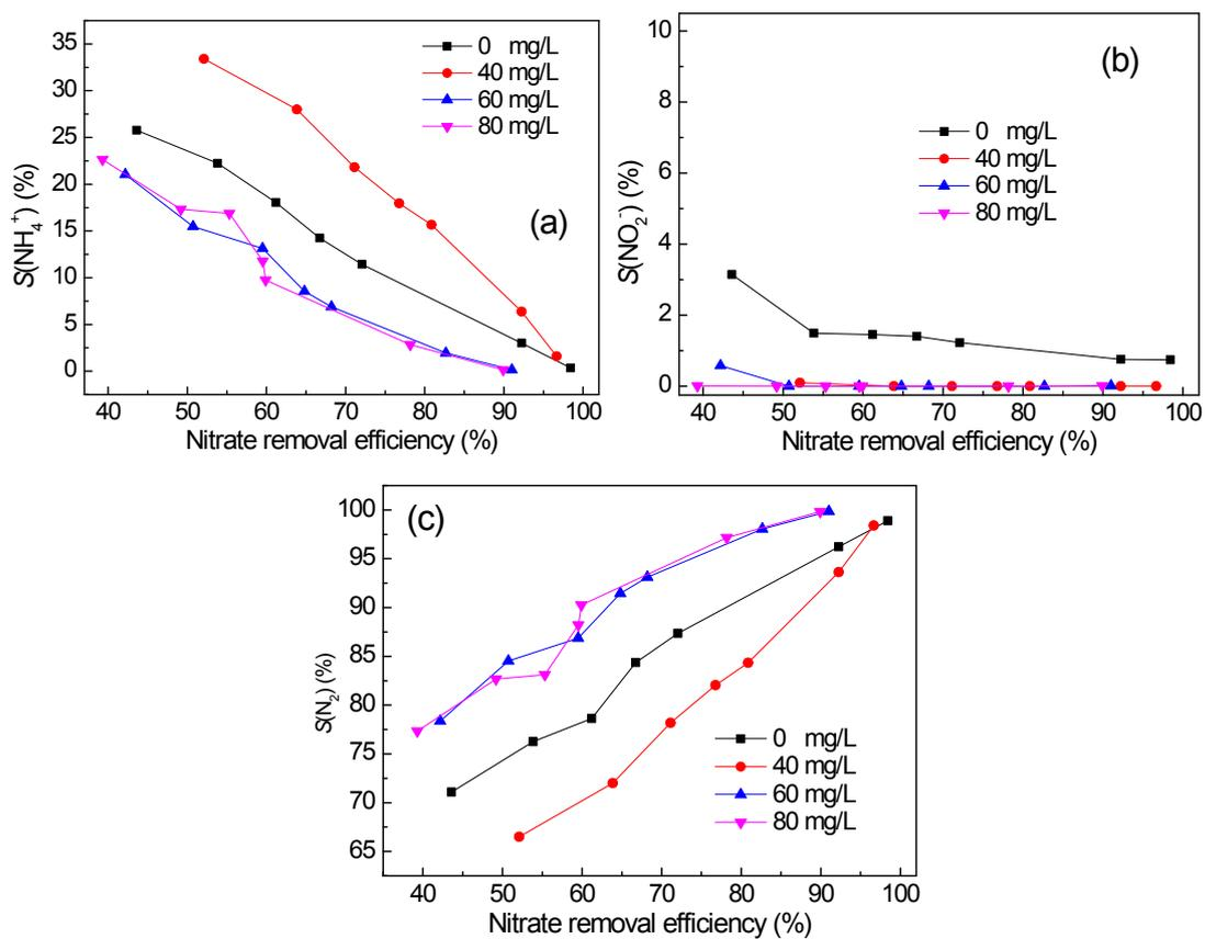
Fig. S3 Product selectivity as a function of nitrate removal efficiency at different concentration of  $\text{HCO}_3^-$ : (a)  $\text{NH}_4^+$ -N; (b)  $\text{NO}_2^-$ -N; (c)  $\text{N}_2$
