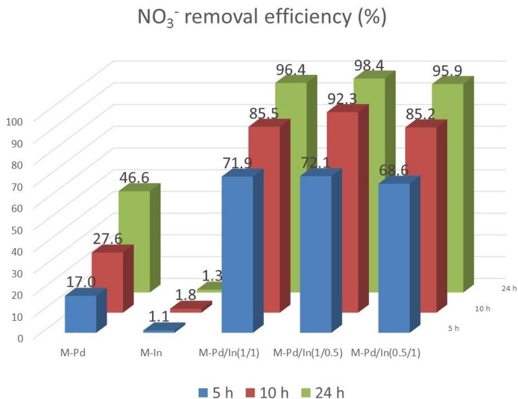
Fig. S1 The  $\text{NO}_3^-$  removal efficiency of the prepared Pd/In bimetallic composites after 5h, 10h and 24h of reaction
