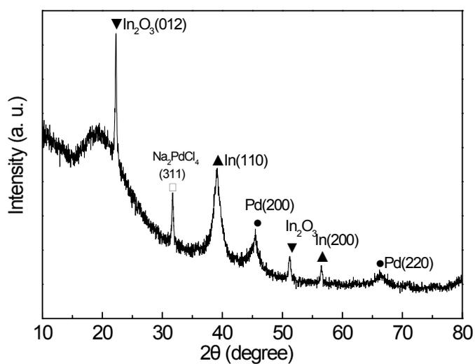
Fig. S13 XRD spectrum of M-Pd/In(1/0.5) after 5 cycles of reuse
