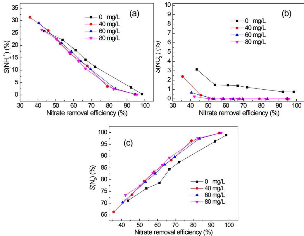
Fig. S4 Product selectivity as a function of nitrate removal efficiency at different concentration of  $\text{Cl}^-$ : (a)  $\text{NH}_4^+\text{-N}$ ; (b)  $\text{NO}_2^-\text{-N}$ ; (c)  $\text{N}_2$
