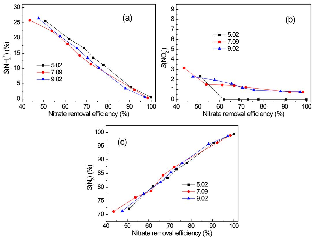
Fig. S7 Product selectivity as a function of nitrate removal efficiency at different initial pH: (a) NH<sub>4</sub><sup>+</sup>-N; (b) NO<sub>2</sub><sup>-</sup>-N; (c) N<sub>2</sub>
