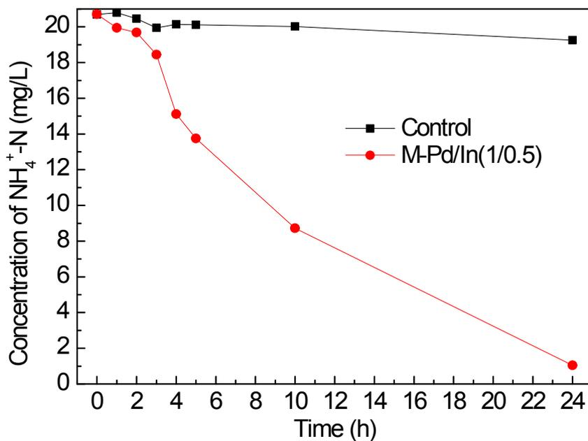
Fig. S9 The concentration of NH<sub>4</sub><sup>+</sup>-N in the presence of M-Pd/In(1/0.5) and the control at the initial pH of 9.50
