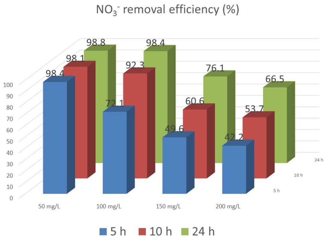
Fig. S2 The  $\text{NO}_3^-$  removal efficiency of M-Pd/In(1/0.5) at the 5<sup>th</sup> hour, the 10<sup>th</sup> hour and the 24<sup>th</sup> hour at the condition of different initial  $\text{NO}_3^-$ -N concentration
