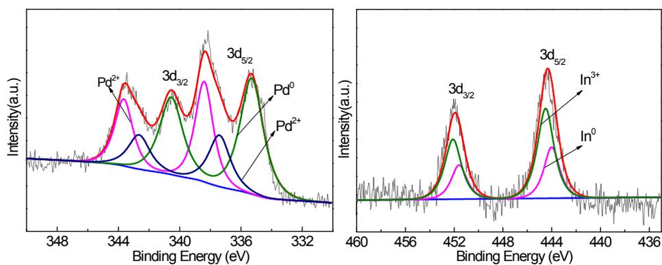
Fig. S14 XPS results of the prepared M-Pd/In composite after 5 cycles of reuse: (a) Pd and (b) In
