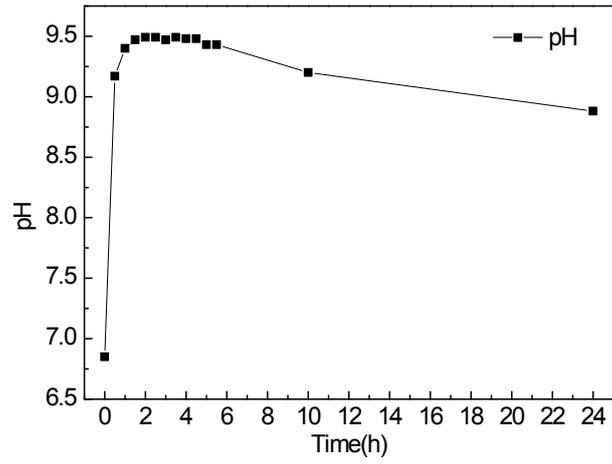
Fig. S10 The pH value during the nitrate removal reaction by M-Pd/In(1/0.5)
