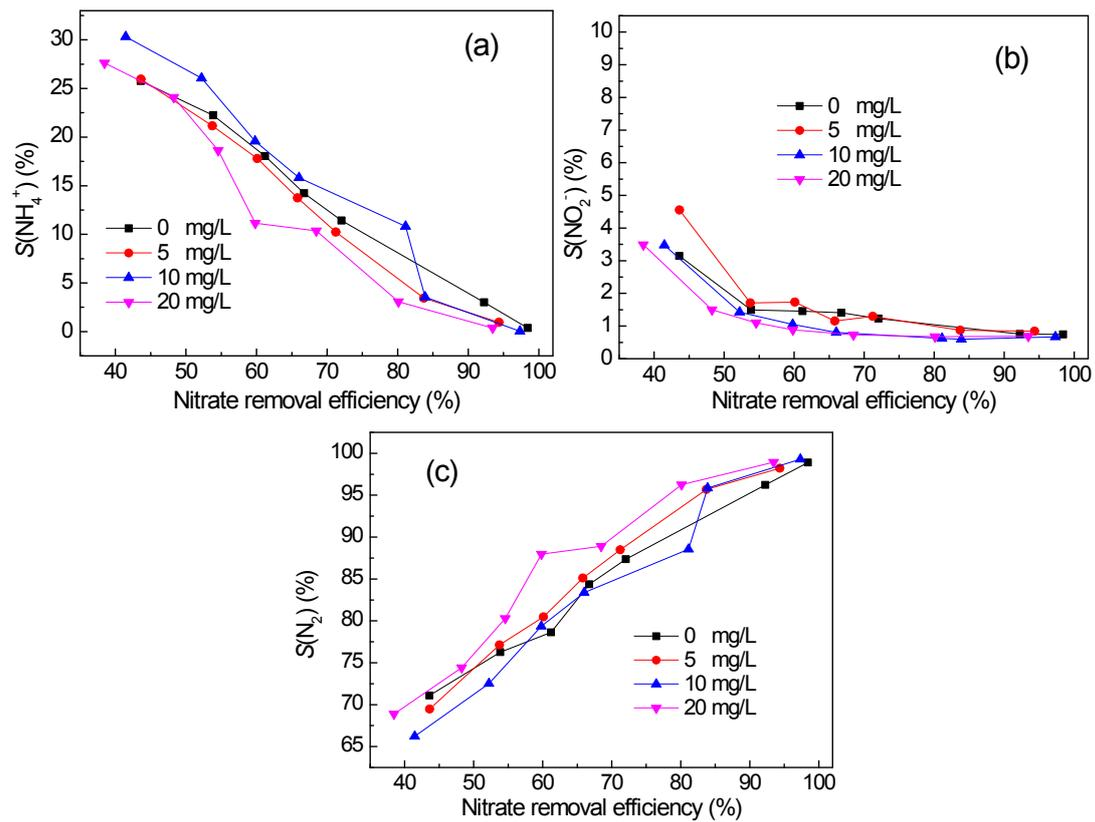
Fig. S6 Product selectivity as a function of nitrate removal efficiency at different concentration of humic acid: (a)  $\text{NH}_4^+$ -N; (b)  $\text{NO}_2^-$ -N; (c)  $\text{N}_2$
