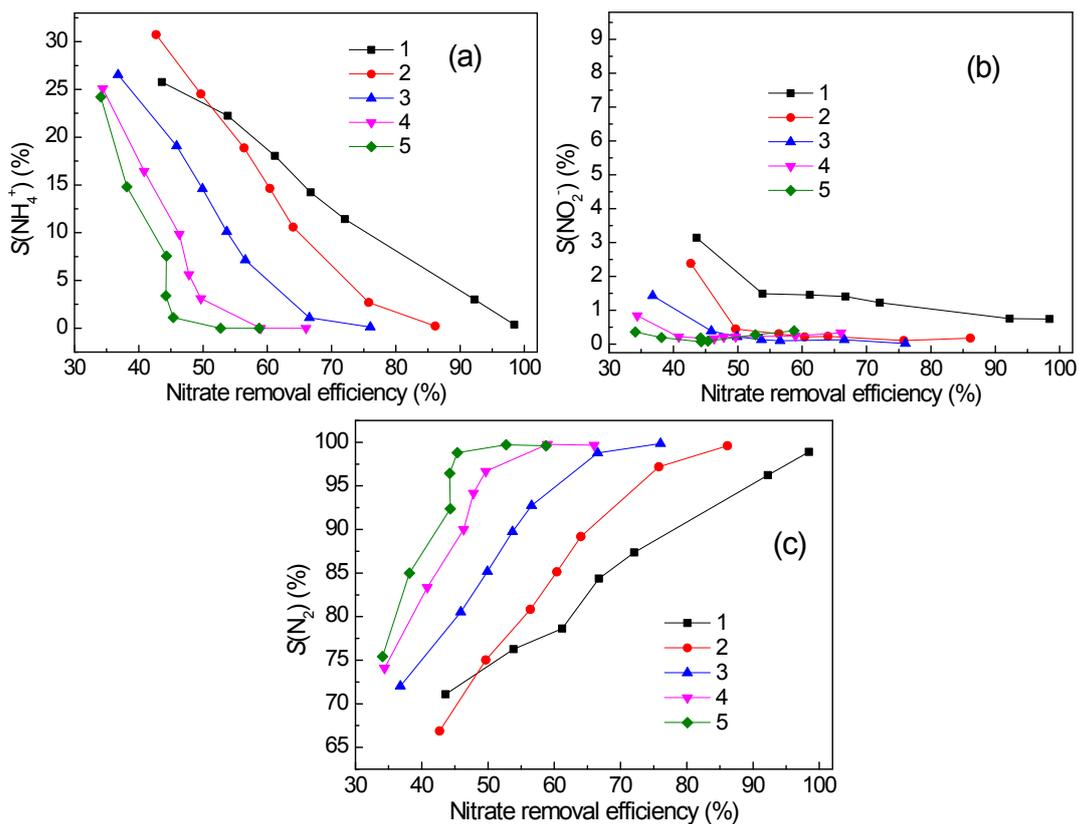
Fig. S8 Product selectivity as a function of nitrate removal efficiency at different recycling nitrate removal reaction (1 to 5): (a) NH<sub>4</sub><sup>+</sup>-N; (b) NO<sub>2</sub><sup>-</sup>-N; (c) N<sub>2</sub>
