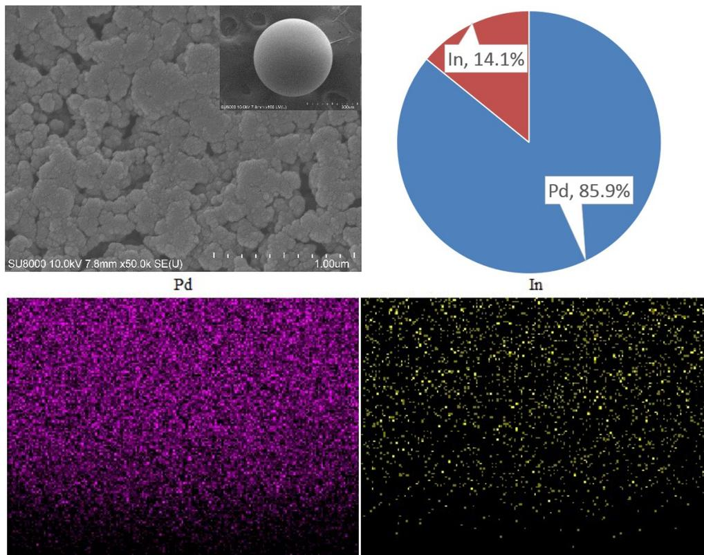
Fig. S11 FESEM-EDS results of M-Pd/In(1/0.5) after 5 cycles of reuse
