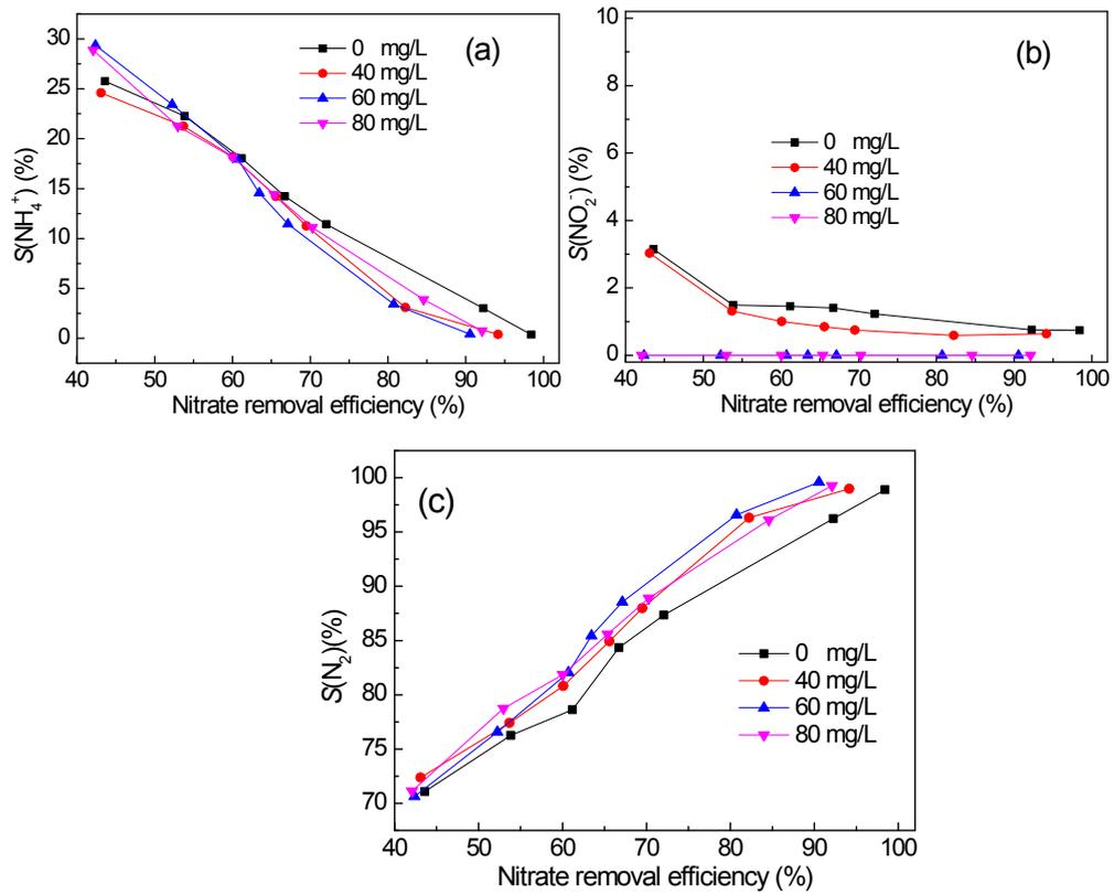
Fig. S5 Product selectivity as a function of nitrate removal efficiency at different concentration of  $\text{SO}_4^{2-}$ : (a)  $\text{NH}_4^+\text{-N}$ ; (b)  $\text{NO}_2^-\text{-N}$ ; (c)  $\text{N}_2$
