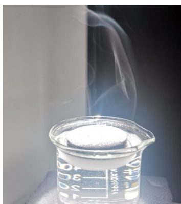
Figure S1. Digital photos of steam generated under 3 solar irradiation of JBCS.
