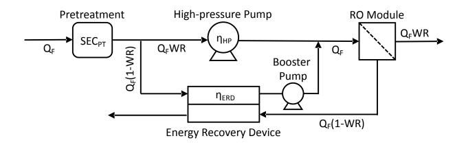
**RO Operating Pressure.** For a single-pass constant-pressure RO, the minimum applied pressure,  $\Delta p_{min}$ , is the osmotic pressure of the existing brine (as a function of *WR*),  $\pi_b(WR)$ .
