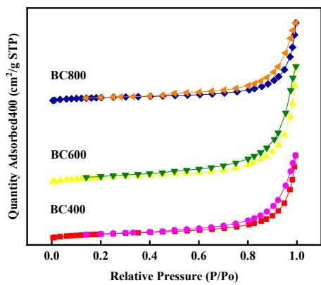
**Fig. S1** The nitrogen adsorption-desorption isotherms of biochar samples in different pyrolysis temperatures.
