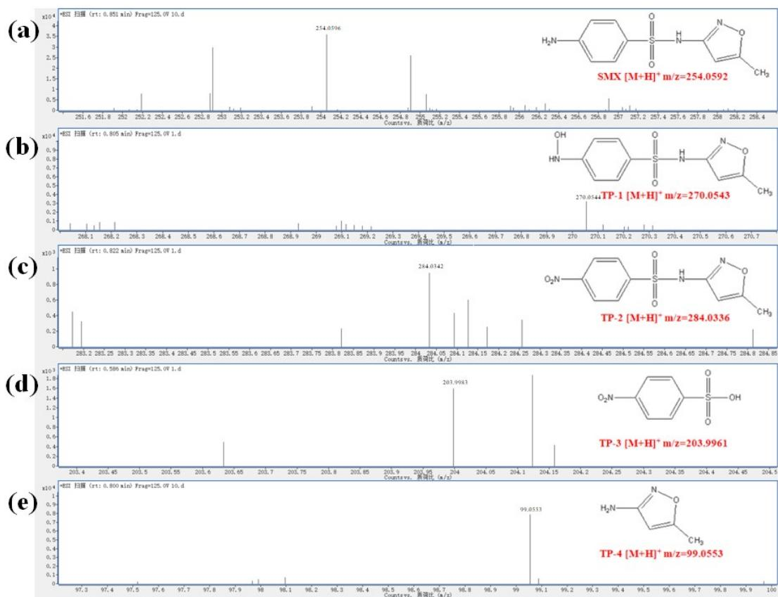
**Fig. S4** SMX and main intermediate products of SMX during the treatment process
