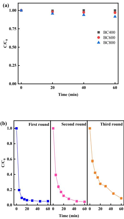
**Fig. S3** The adsorption capacity of biochar samples **(a)**; stability and reusability of BC800 for the degradation of SMX **(b)**. Conditions:  $[SMX] = 10 \mu M$ ,  $[PDS] = 1 mM$ ,  $[BC800] = 0.75 g L^{-1}$ , initial pH=7.0, T=25 °C.
