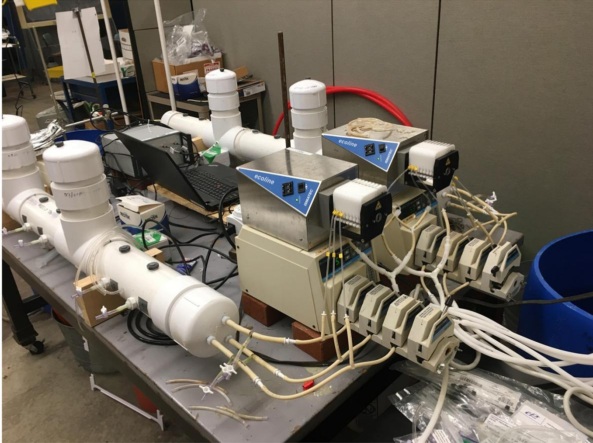
Figure S2: Image of laboratory flow-through reactor. Peristaltic pumps for flow control are seen in the foreground. Reactor sampling ports can be visualized on the left-side of the reactor seen in the left-hand side of the photograph. Dissolved oxygen probes are located at the junction of the reactor barrel and woodchip sampling ports. In this photograph, flow through the reactors proceeds from the lower right to the upper left.
