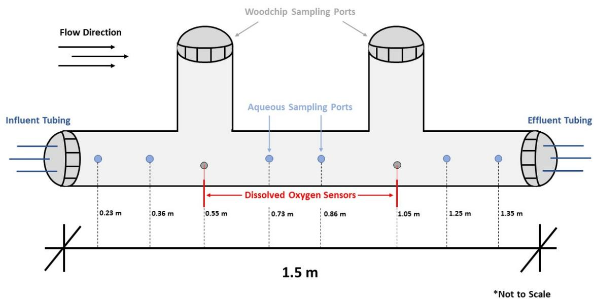
Figure S1: Schematic of a single flow-through reactor.
